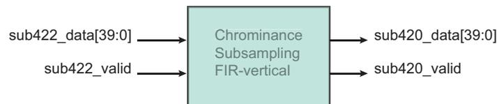
The SUB420 module samples the sub422\_data[39:0] 40-bit data when sub422\_valid is asserted, then it performs a vertical subsampling and generates a valid sub420\_data[39:0] 40-bit word and the corresponding sub420\_valid signal.
