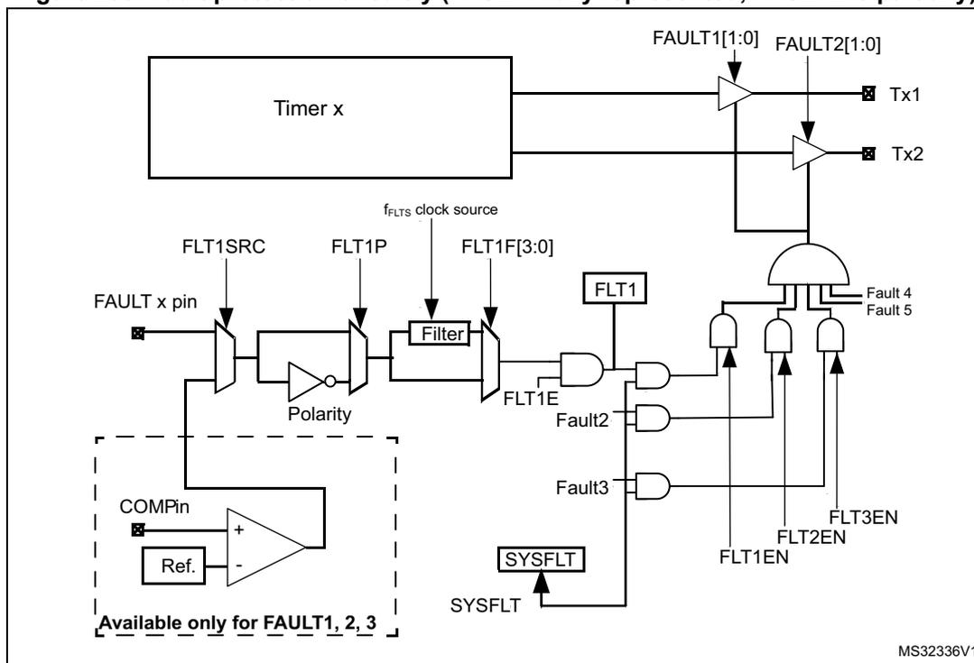
Each fault channel is fully configurable using HRTIM\_FLTINR1 and HRTIM\_FLTINR2 registers before being routed to the timing units. FLT<sub>x</sub>SRC bit selects the source of the Fault signal, that can be either a digital input or an internal event (built-in comparator output).
