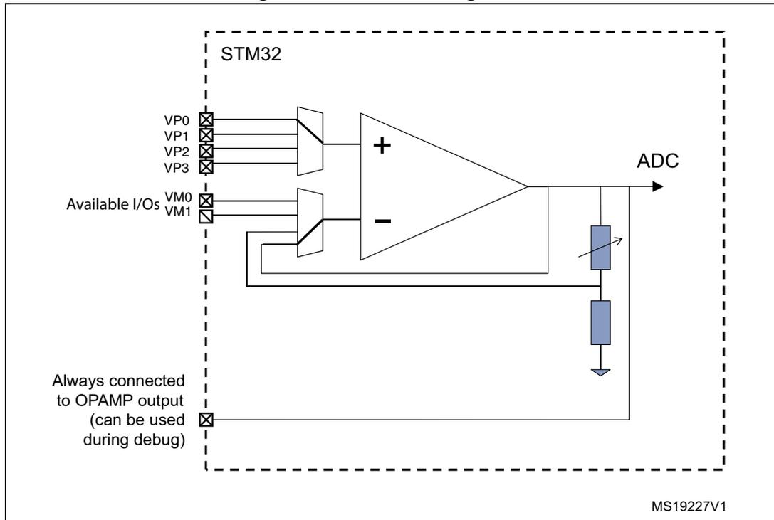
1. This figure gives an example in an inverting configuration. Any other option is possible, including comparator mode.
