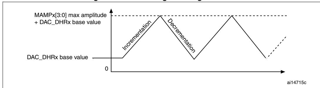
**Figure 91. DAC conversion (SW trigger enabled) with triangle wave generation**
