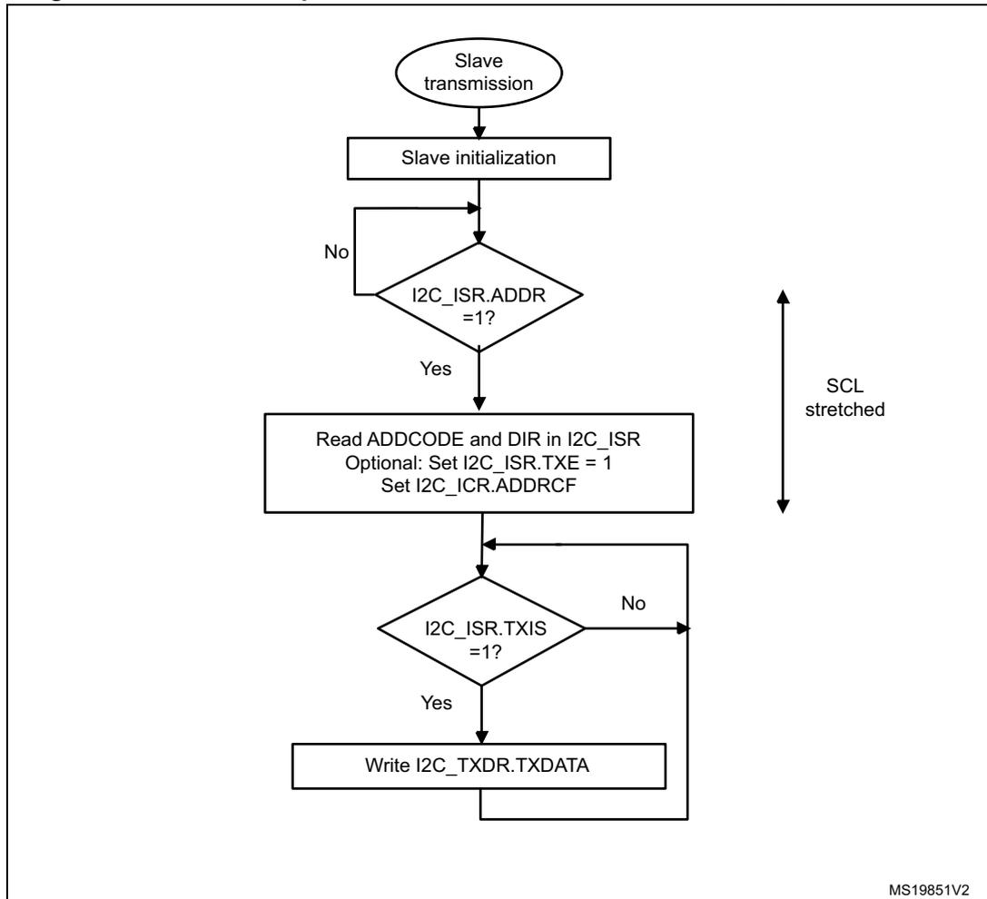
Figure 332. Transfer sequence flowchart for I2C slave transmitter, NOSTRETCH=1
