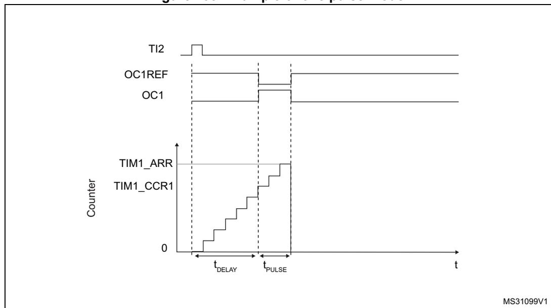
For example you may want to generate a positive pulse on OC1 with a length of  $t_{PULSE}$  and after a delay of  $t_{DELAY}$  as soon as a positive edge is detected on the TI2 input pin.
