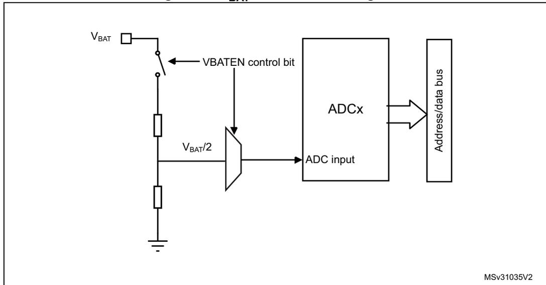
Note: The VBATEN bit must be set to enable the conversion of internal channel ADC1\_IN17 ( $V_{BATEN}$ ).
