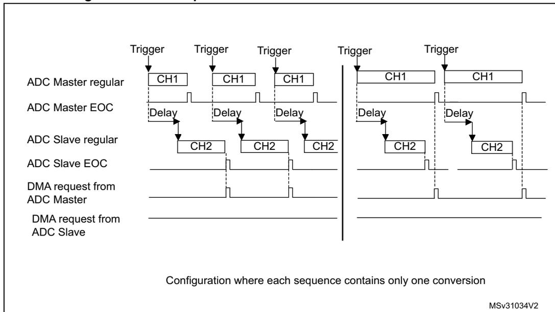
*Note:* When using MDMA mode, the user must take care to configure properly the duration of the master and slave conversions so that a DMA request is generated and served for reading both data (master + slave) before a new conversion is available.
