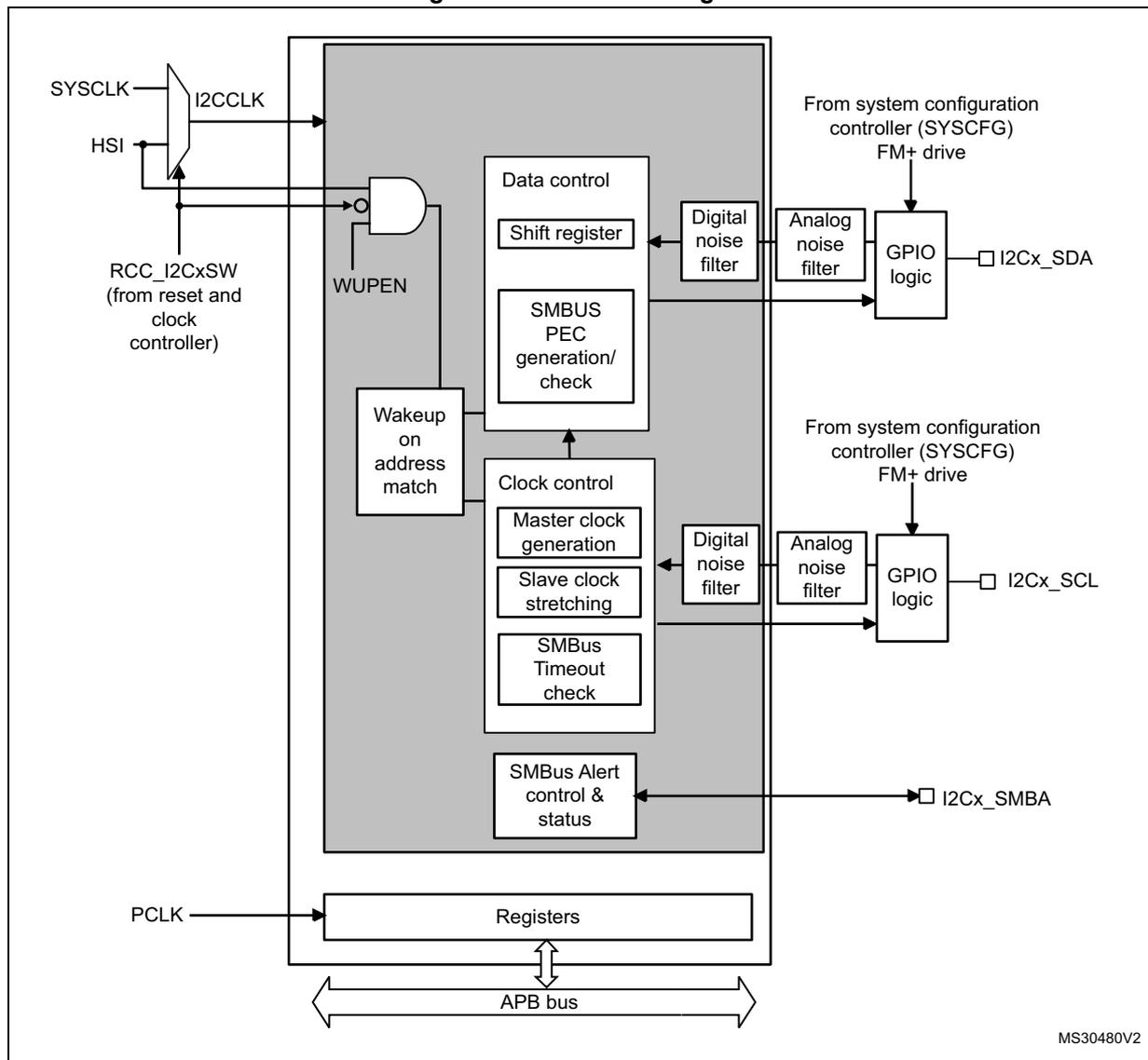
The I2C is clocked by an independent clock source which allows to the I2C to operate independently from the PCLK frequency.
