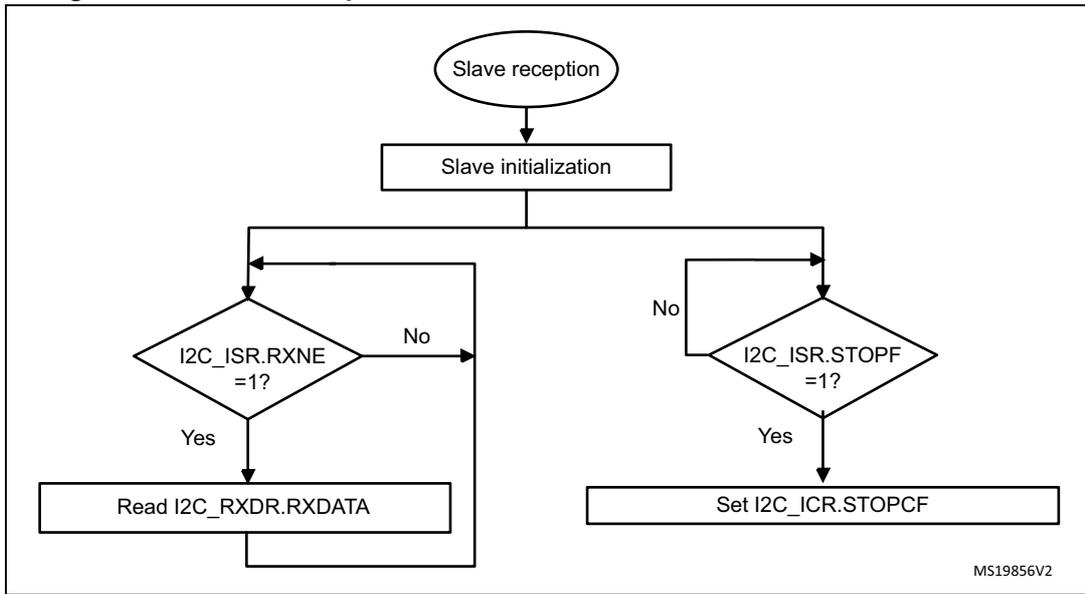
Figure 336. Transfer bus diagrams for I2C slave receiver
