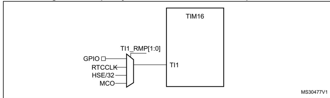
The input capture channel of the Timer 16 can be a GPIO line or an internal clock of the MCU. This selection is performed through the T11\_RMP [1:0] bits in the TIM16\_OR register. The possibilities available are the following ones.
