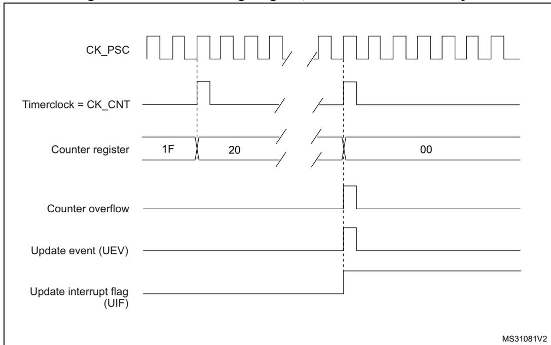
**Figure 112. Counter timing diagram, update event when ARPE=0 (TIMx\_ARR not preloaded)**
