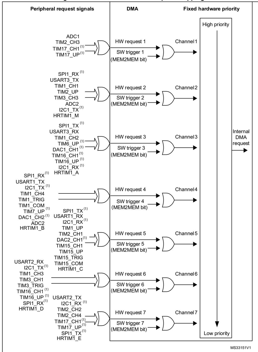
1. DMA request are mapped on this DMA channel only if the corresponding remapping bit is set in the SYSCFG\_CFGR1 or SYSCFG\_CFGR3 register. For more details, please refer to [Section 10.1.1: SYSCFG configuration register 1 \(SYSCFG\\_CFGR1\)](#) and [Section 10.1.8: SYSCFG configuration register 3 \(SYSCFG\\_CFGR3\)](#).
