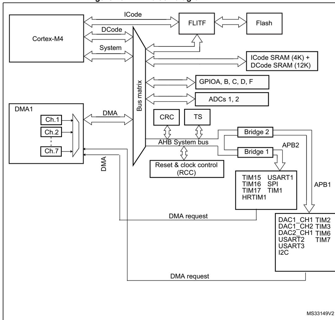
The DMA controller performs direct memory transfer by sharing the system bus with the Arm® Cortex®-M4 core. The DMA request may stop the CPU access to the system bus for some bus cycles, when the CPU and DMA are targeting the same destination (memory or peripheral). The bus matrix implements round-robin scheduling, thus ensuring at least half of the system bus bandwidth (both to memory and peripheral) for the CPU.
