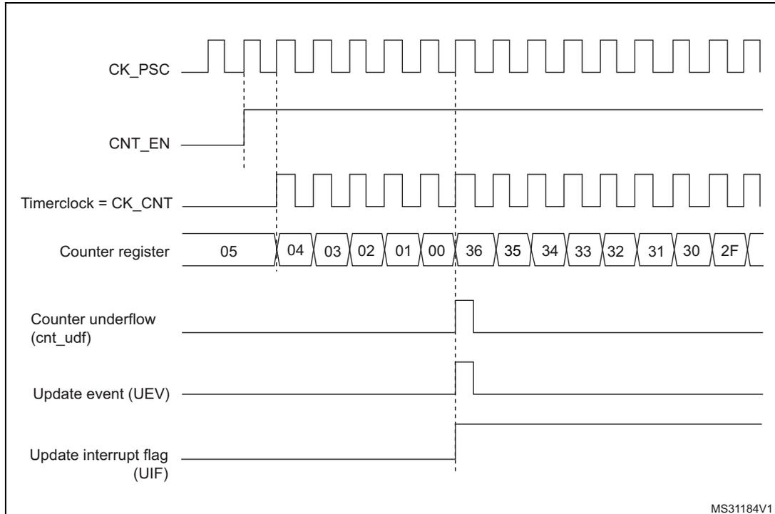
**Figure 173. Counter timing diagram, internal clock divided by 2**
