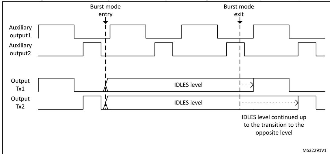
The signal on the auxiliary output can be slightly distorted when exiting from the burst mode or when re-enabling the outputs after a delayed protection, if this happens during a deadtime. In this case, the deadtime applied to the auxiliary outputs is extended so that the deadtime on the main outputs is respected. [Figure 294](#) gives some examples.
