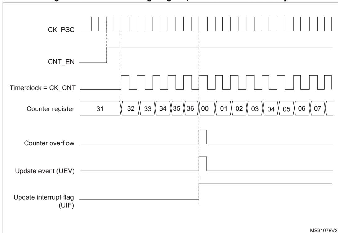
Figure 314. Counter timing diagram, internal clock divided by 2
