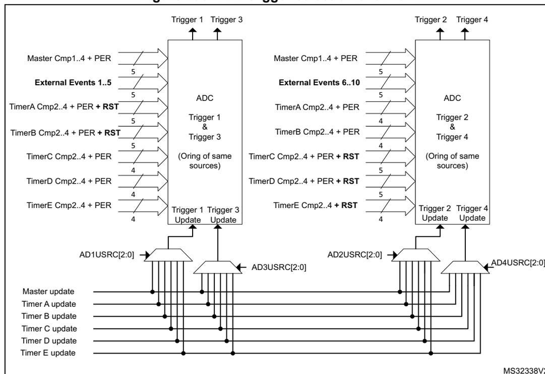
HRTIM\_ADC1R to HRTIM\_ADC4R registers are preloaded and can be updated synchronously with the timer they are related to. The update source is defined with ADxUSRC[2:0] bits in the HRTIM\_CR1 register.
