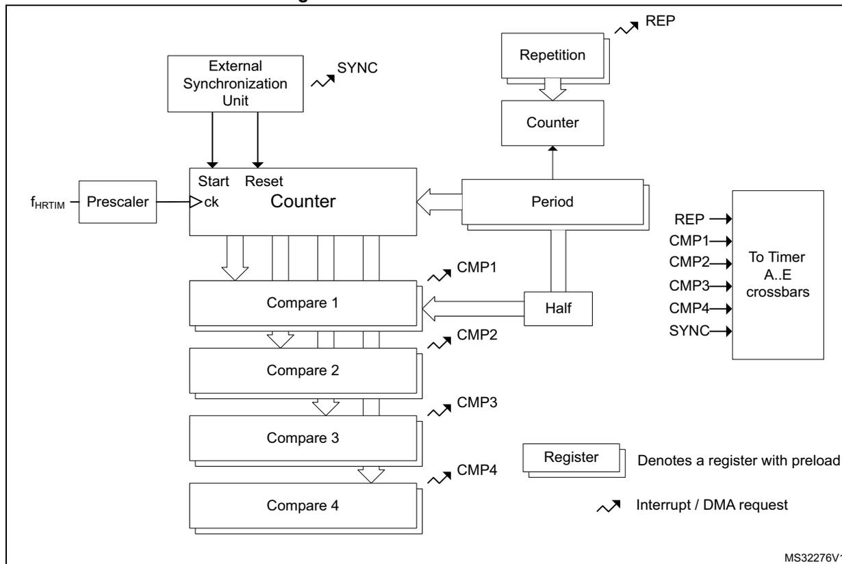
The master timer is based on the very same architecture as the timing units, with the following differences:
