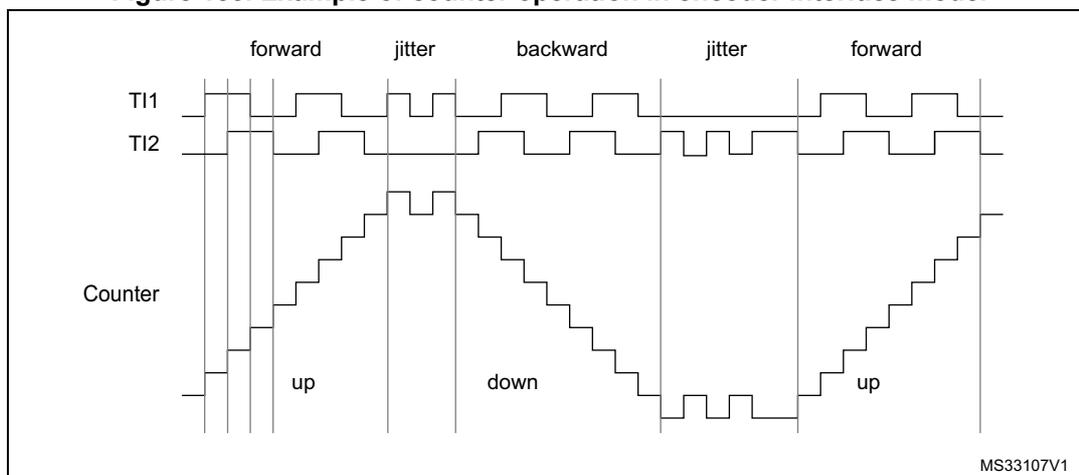
Figure 156 gives an example of counter behavior when TI1FP1 polarity is inverted (same configuration as above except CC1P='1').
