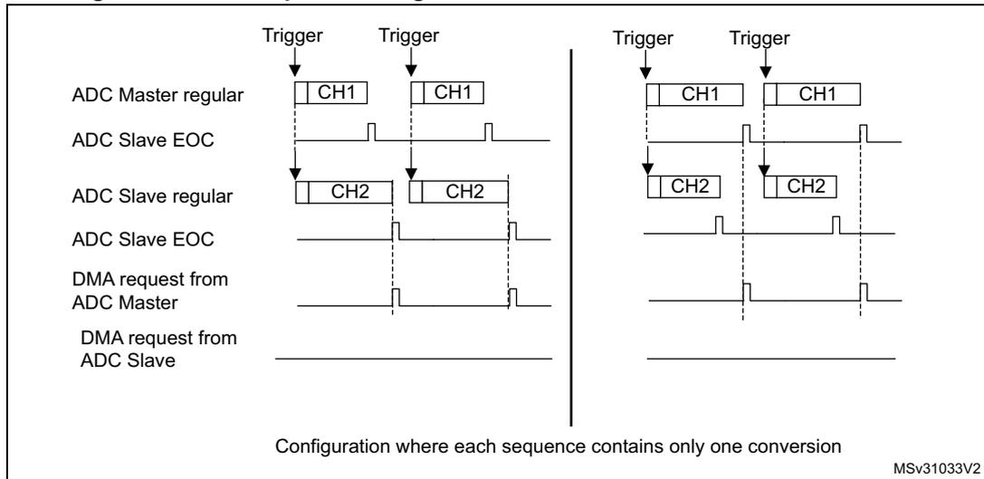
Figure 79. DMA requests in interleaved mode when MDMA=0b10
