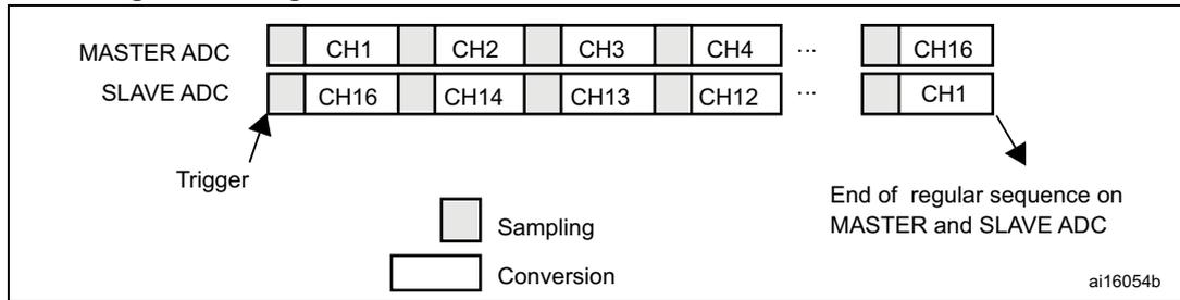
If DISCEN=1 then each “n” simultaneous conversions of the regular sequence require a regular trigger event to occur (“n” is defined by DISCNUM).
