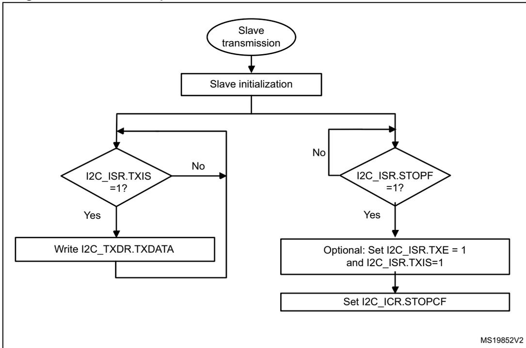
Figure 333. Transfer bus diagrams for I2C slave transmitter
