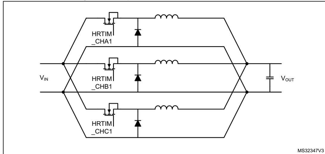
The master timer is responsible for the phase management: it defines the phase relationship between the converters by resetting the timers periodically. The phase-shift is  $360^\circ$  divided by the number of phases,  $120^\circ$  in the given example.
