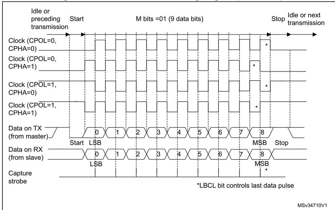
Figure 369. RX data setup/hold time
