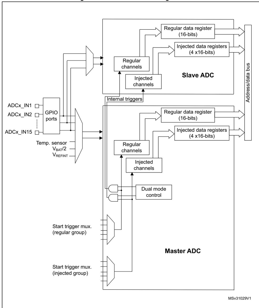
1. External triggers also exist on slave ADC but are not shown for the purposes of this diagram.
