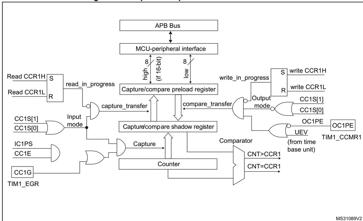
Figure 228. Output stage of capture/compare channel (channel 1)
