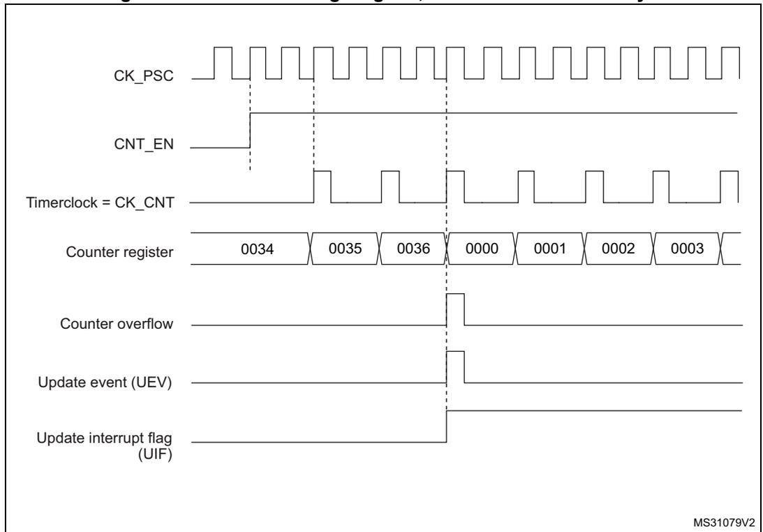
Figure 218. Counter timing diagram, internal clock divided by 4
