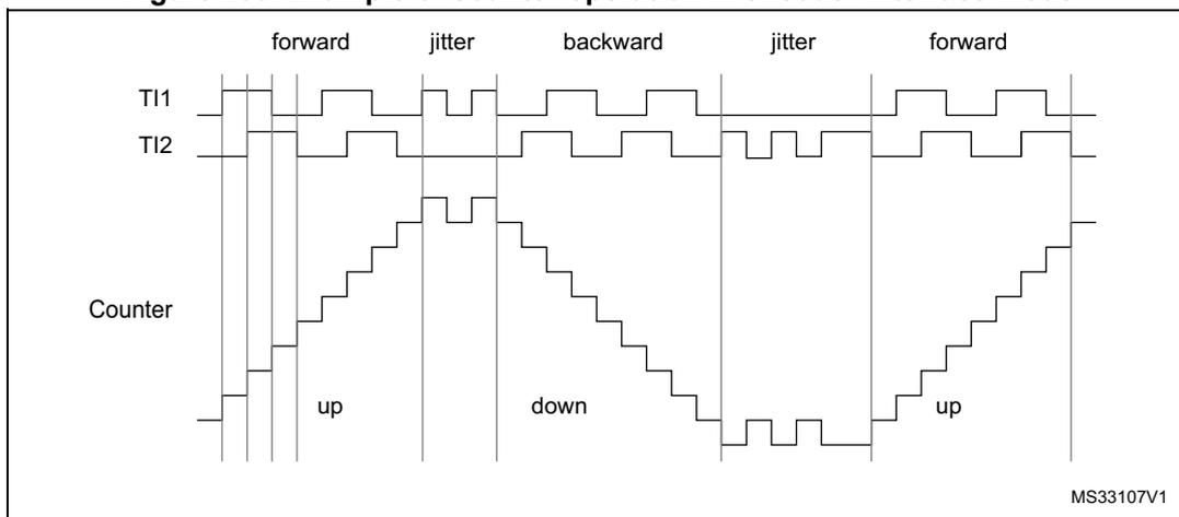
Figure 201 gives an example of counter behavior when TI1FP1 polarity is inverted (same configuration as above except CC1P=1).
