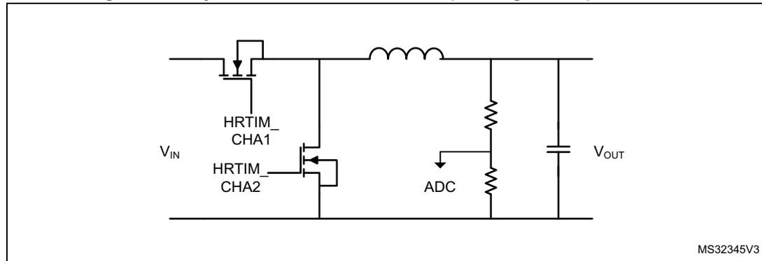
The main difference vs. a single-switch buck converter is the addition of a deadtime for an almost complementary waveform generation on HRTIM\_CHA2, based on the reference waveform on HRTIM\_CHA1 (see [Figure 304](#)).
