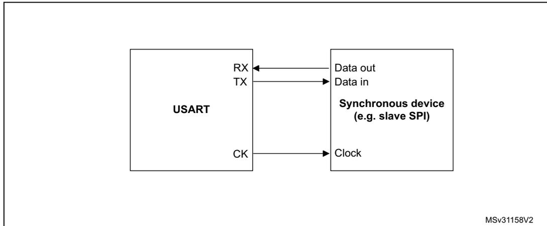
**Figure 367. USART data clock timing diagram (M bits = 00)**
