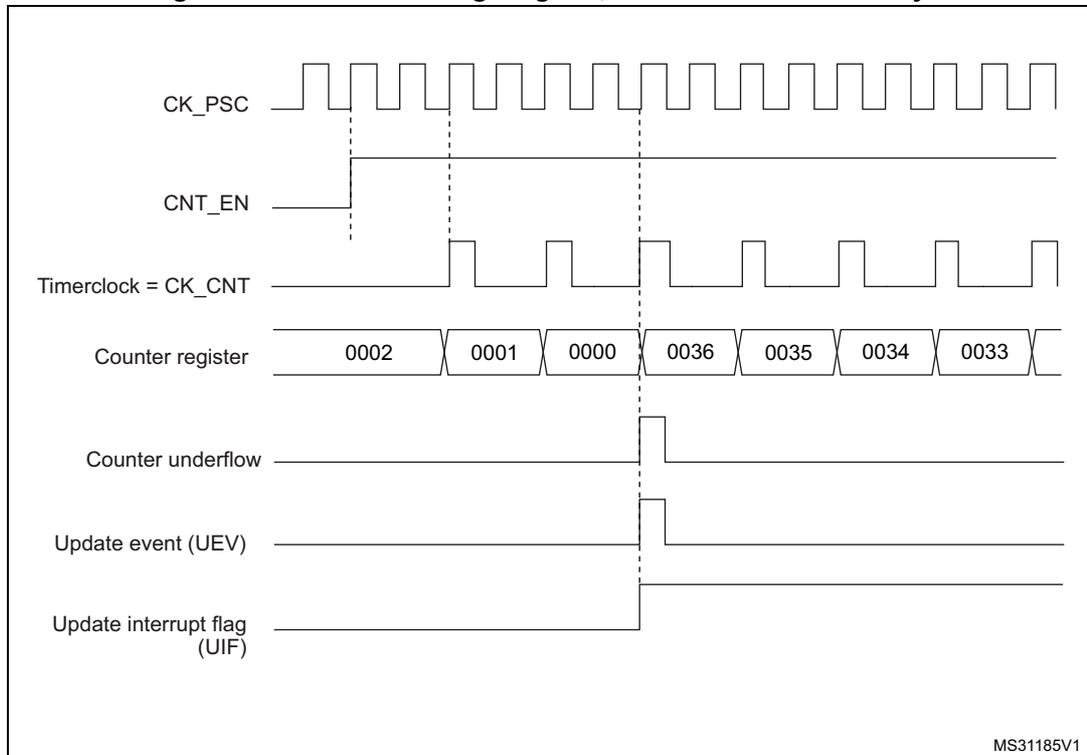
Figure 174. Counter timing diagram, internal clock divided by 4
