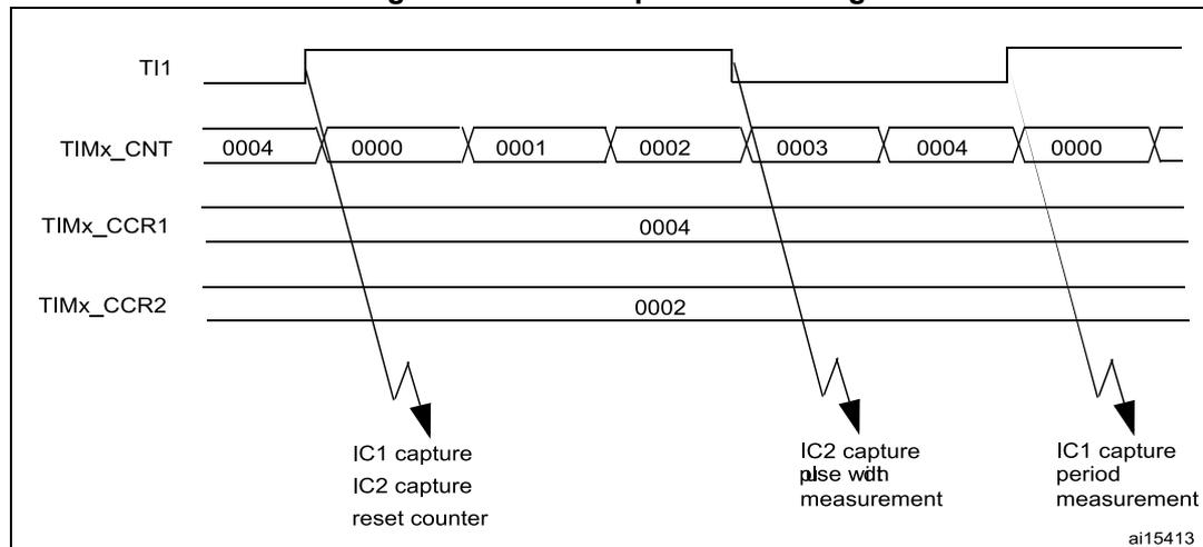
1. The PWM input mode can be used only with the TIMx\_CH1/TIMx\_CH2 signals due to the fact that only TI1FP1 and TI2FP2 are connected to the slave mode controller.
