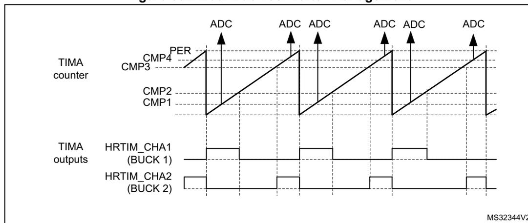
Timers A..E provide either 10 buck converters coupled by pairs (both with identical switching frequencies) or 6 completely independent converters (each of them having a different switching frequency), using the master timer as the 6<sup>th</sup> time base.
