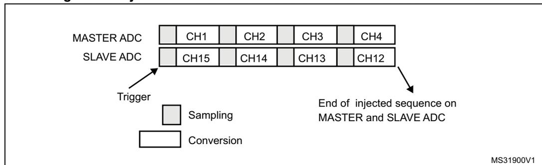
If JDISCEN=1, each simultaneous conversion of the injected sequence requires an injected trigger event to occur.
