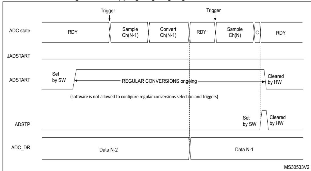
Figure 32. Stopping ongoing regular and injected conversions
