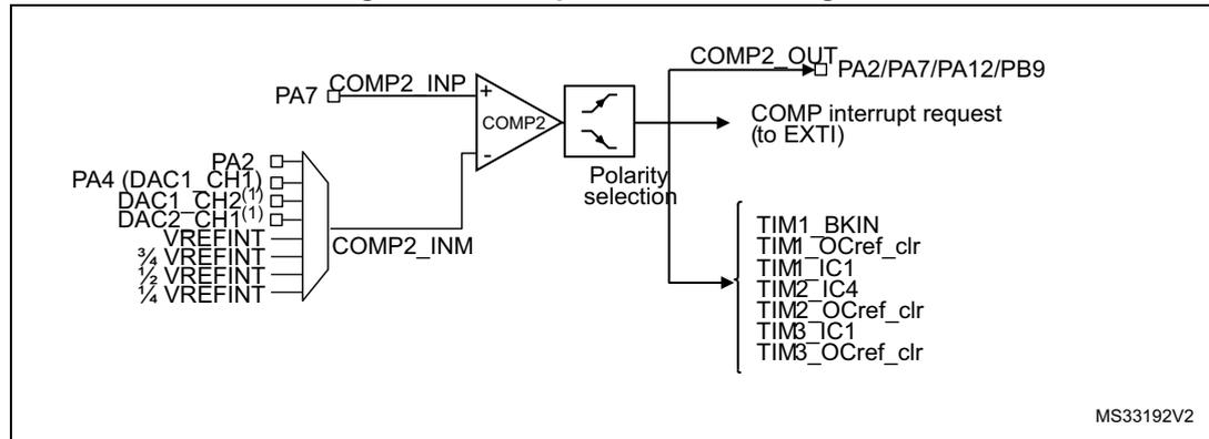
1. In STM32F334xx devices, DAC1\_CH2 and DAC2\_CH1 outputs are connected directly, thus PA5 and PA6 are not available as COMP2\_INM inputs.
