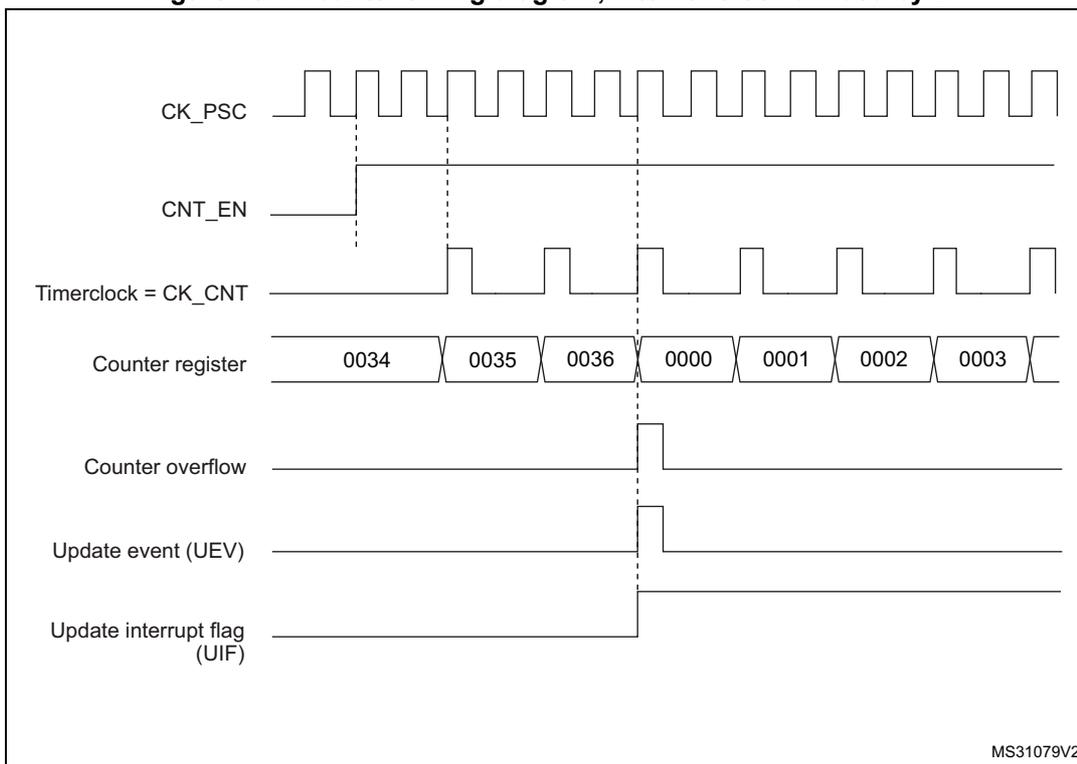
Figure 168. Counter timing diagram, internal clock divided by 4
