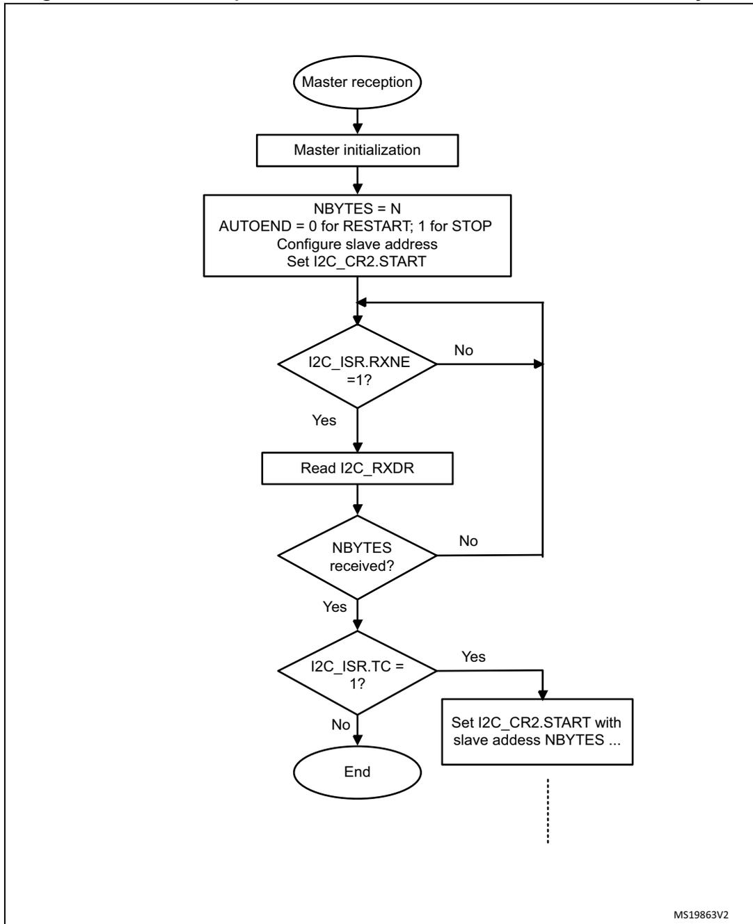
Figure 345. Transfer sequence flowchart for I2C master receiver for N >255 bytes
