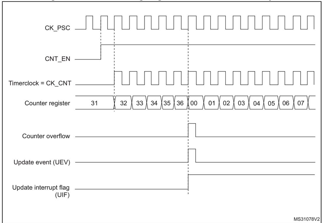
**Figure 109. Counter timing diagram, internal clock divided by 2**
