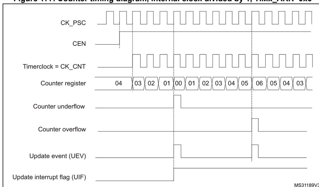
1. Here, center-aligned mode 1 is used (for more details refer to [Section 19.4.1: TIMx control register 1 \(TIMx\\_CR1\) on page 525](#)).
