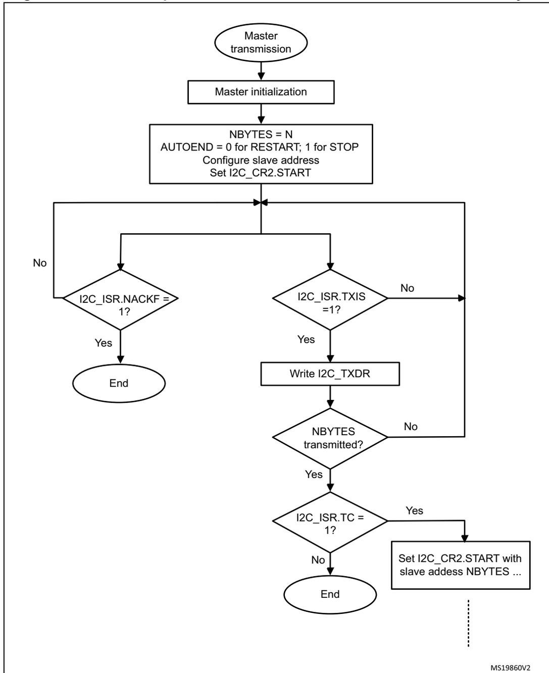
Figure 342. Transfer sequence flowchart for I2C master transmitter for N>255 bytes
