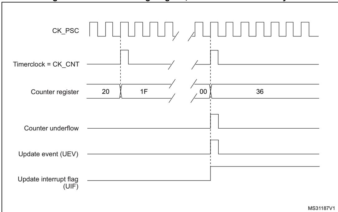
**Figure 118. Counter timing diagram, update event when repetition counter is not used**
