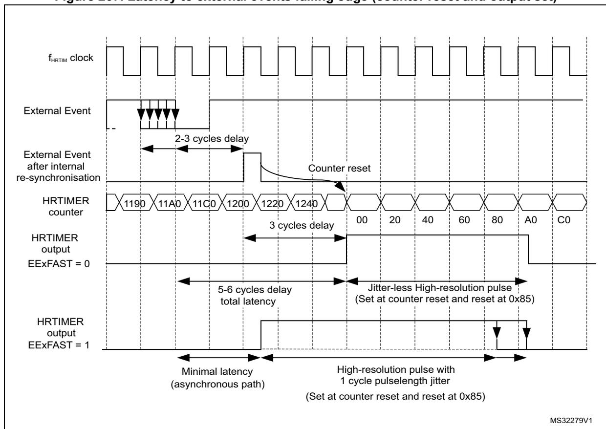
**Figure 268. Latency to external events (output reset on external event)**
