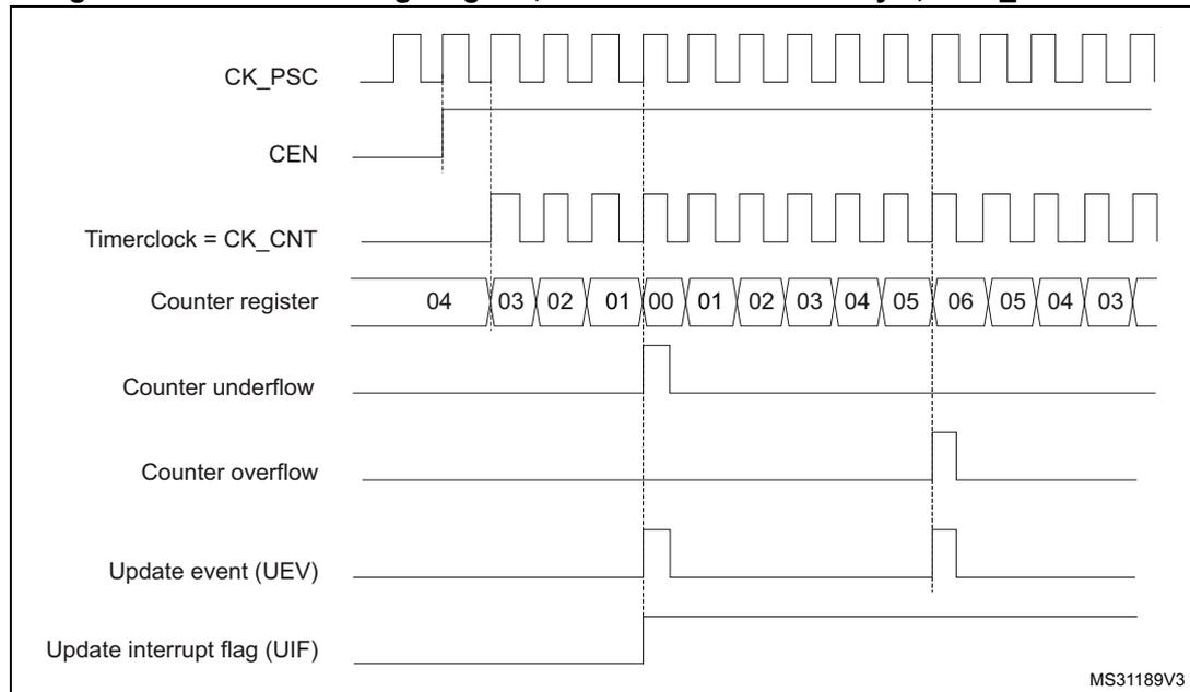
1. Here, center-aligned mode 1 is used (for more details refer to [Section 18.4: TIM1 registers](#)).
