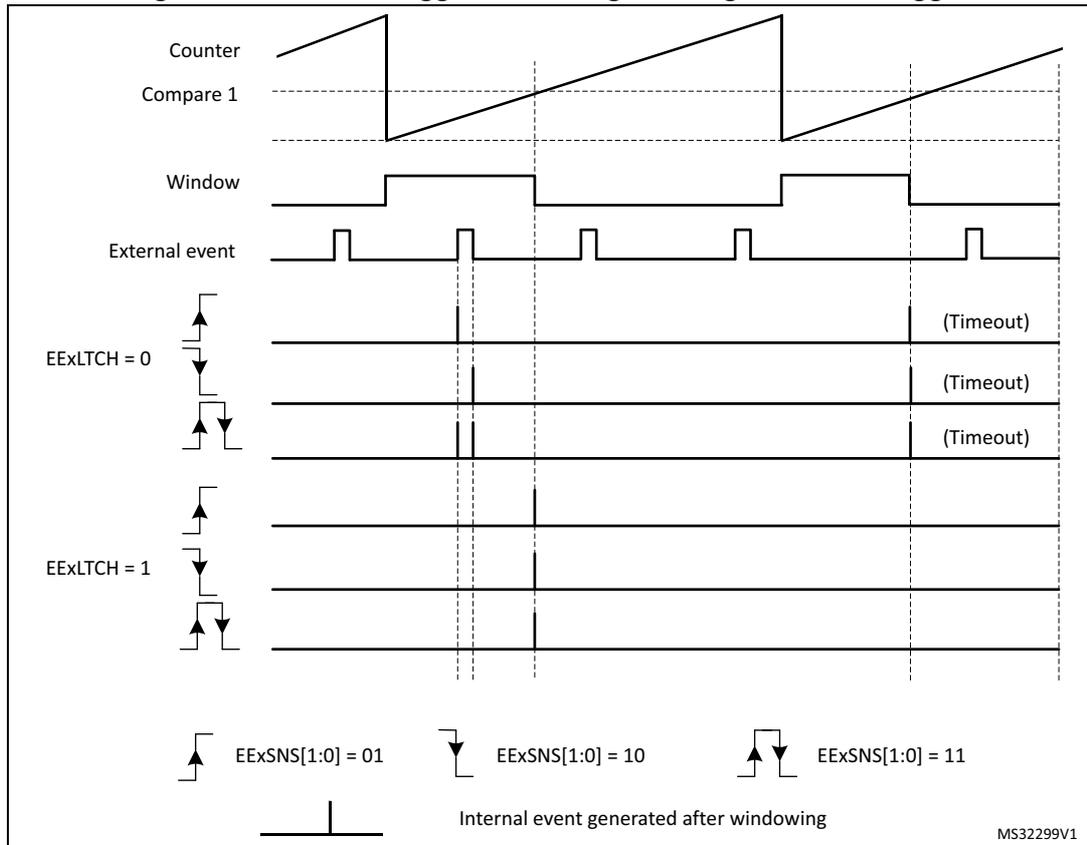
Figure 275. External trigger windowing, level sensitive triggering
