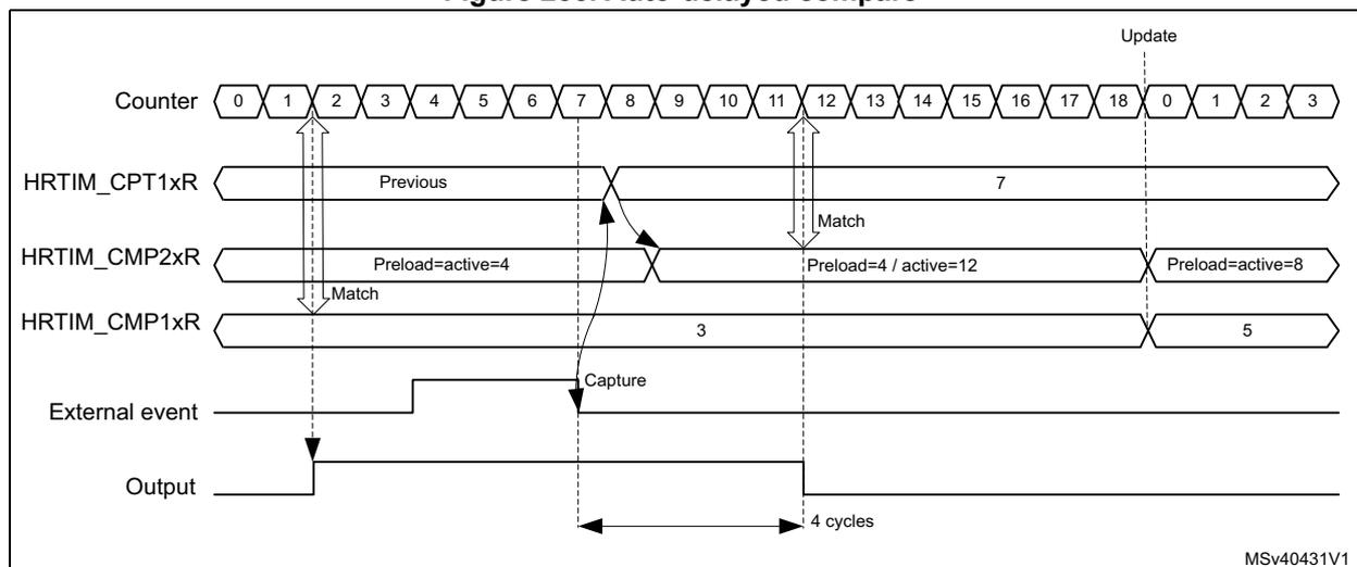
A regular compare channel (e.g. Compare 1) is used for the output set: as soon as the counter matches the content of the compare register, the output goes to its active state.
