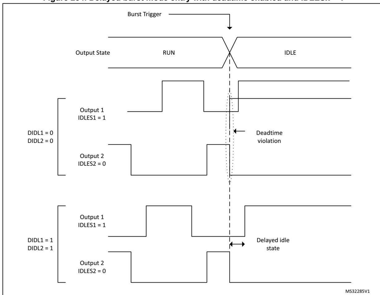
The delayed burst entry mode is enabled with DIDLx bit in the HRTIM\_OUTxR register (one enable bit per output). It forces a deadtime insertion before the output takes its idle state. Each TIMx output has its own deadtime value:
