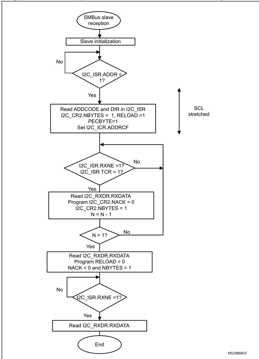
Figure 351. Bus transfer diagrams for SMBus slave receiver (SBC=1)
