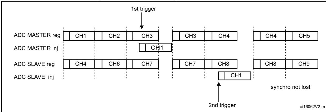
If a trigger occurs during an injected conversion that has interrupted a regular conversion, the alternate trigger is served. [Figure 76](#) shows the behavior in this case (note that the 6th trigger is ignored because the associated alternate conversion is not complete).
