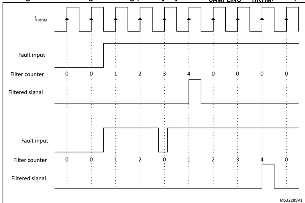
The filtering period ranges from 2 cycles of the  $f_{\text{HRTIM}}$  clock up to 8 cycles of the  $f_{\text{FLTS}}$  clock divided by 32.  $f_{\text{FLTS}}$  is defined using FLTSD[1:0] bits in the HRTIM\_FLTINR2 register. [Table 101](#) summarizes the sampling rate and the filter length. A jitter of 1 sampling clock period must be subtracted from the filter length to take into account the uncertainty due to the sampling and have the effective filtering.
