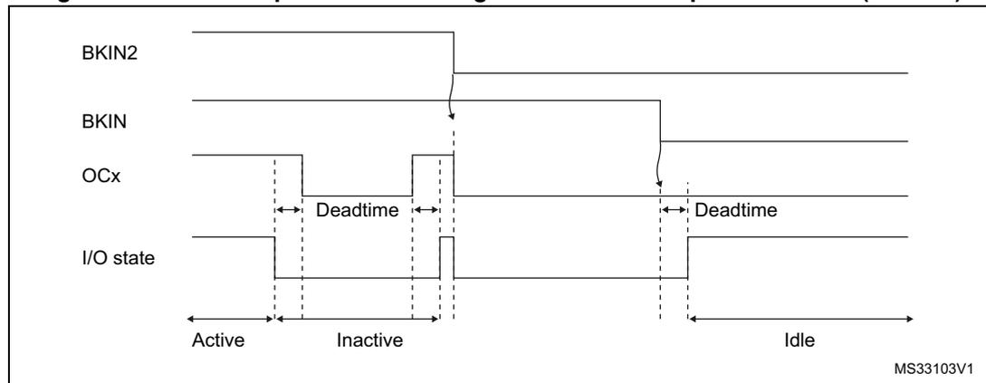
Figure 150. PWM output state following BKIN assertion (OSSI=0)
