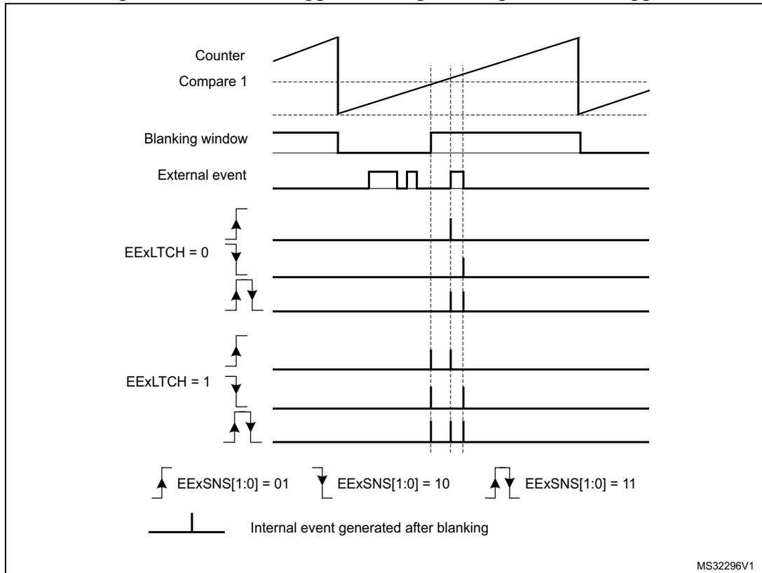
Figure 272. External trigger blanking, level sensitive triggering
