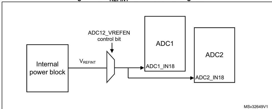
Note: The VREFEN bit into ADC12\_CCR register must be set to enable the conversion of internal channels ADC1\_IN18 or ADC2\_IN18 ( $V_{REFINT}$ ).
