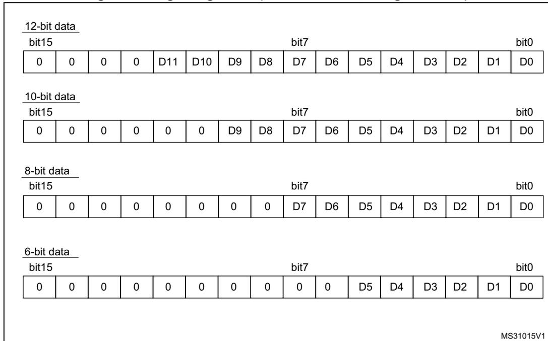
**Figure 53. Right alignment (offset enabled, signed value)**
