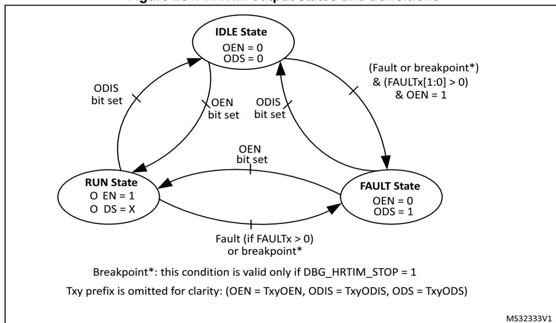
The FAULT and IDLE levels are defined as active or inactive. Active (or inactive) refers to the level on the timer output that causes a power switch to be closed (or opened for an inactive state).
