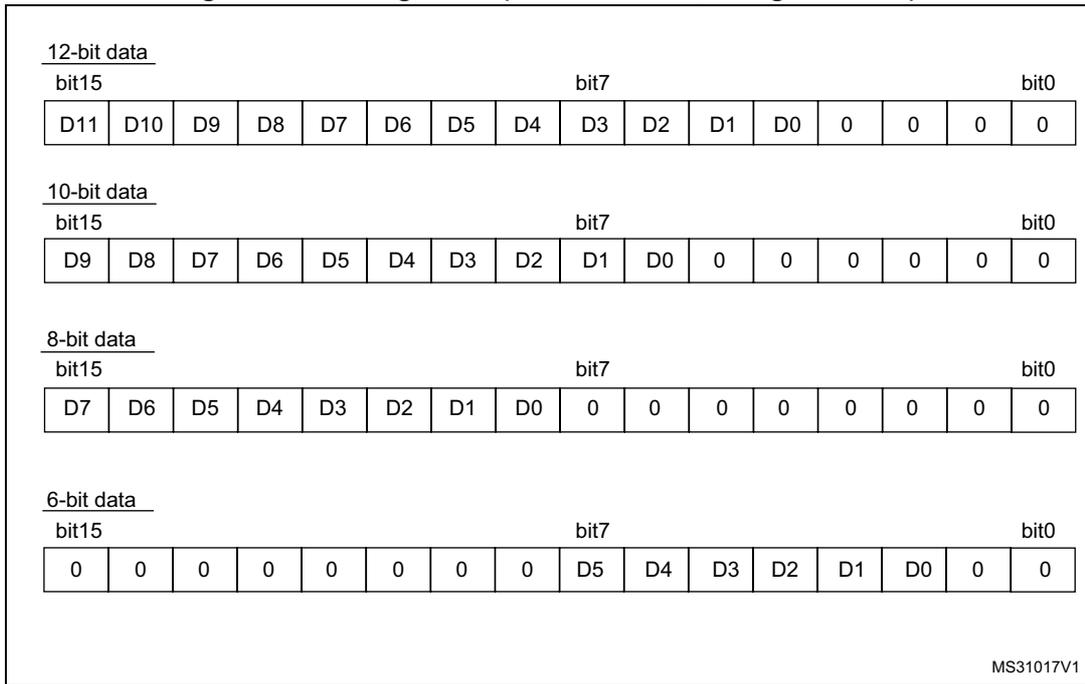
**Figure 55. Left alignment (offset enabled, signed value)**
