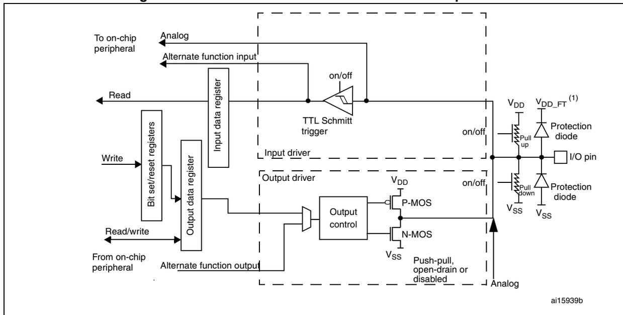
1.  $V_{DD\_FT}$  is a potential specific to five-volt tolerant I/Os and different from  $V_{DD}$ .
