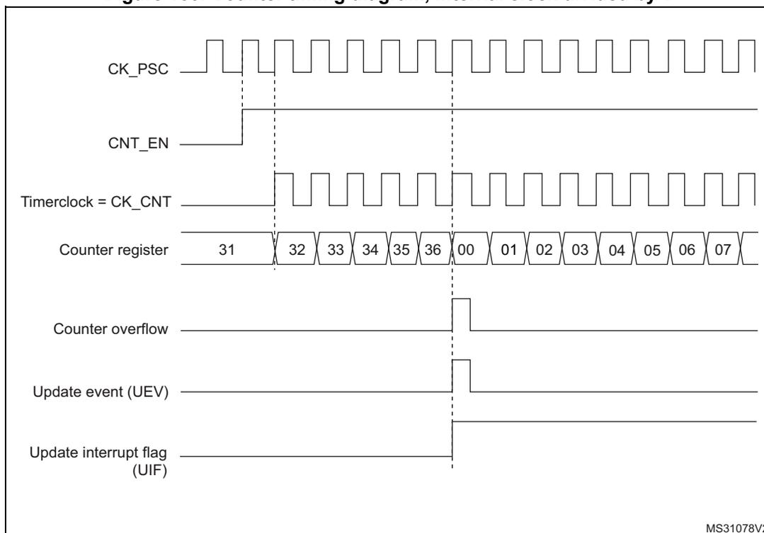
Figure 167. Counter timing diagram, internal clock divided by 2
