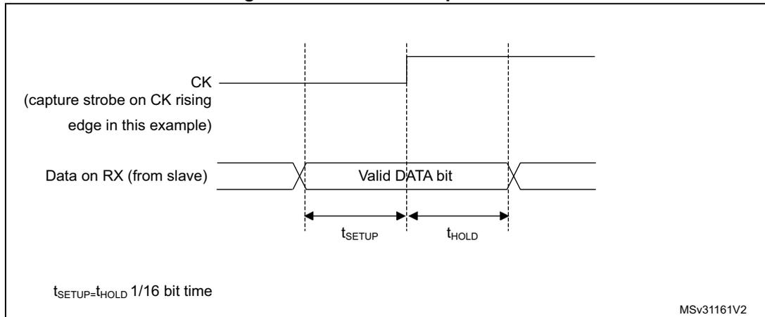
Note: The function of CK is different in Smartcard mode. Refer to [Section 28.5.13: USART Smartcard mode](#) for more details.
