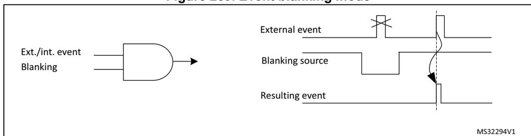
In event postpone mode, the external event is not taken into account immediately but is memorized (latched) and generated as soon as the blanking period is completed, as shown on [Figure 270](#). This mode is enabled by setting EExLTCH bit in HRTIM\_EEFxR1 and HRTIM\_EEFxR2 registers.
