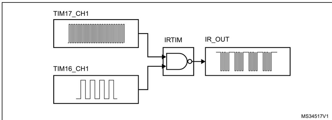
All standard IR pulse modulation modes can be obtained by programming the two timer output compare channels.
