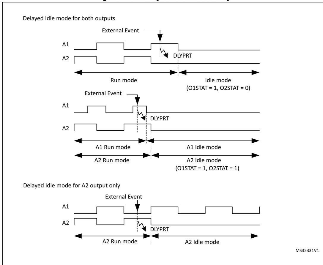
The delayed idle mode has a higher priority than the burst mode: any burst mode exit request is discarded once the delayed idle protection has been triggered. On the contrary, if the delayed protection is exited while the burst mode is active, the burst mode will be resumed normally and the output will be maintained in the idle state until the burst mode exits. [Figure 277](#) gives an overview of these different scenarios.
