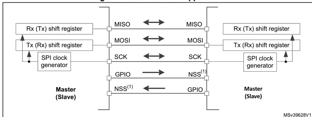
1. The NSS pin is configured at hardware input mode at both nodes. Its active level enables the MISO line output control as the passive node is configured as a slave.
