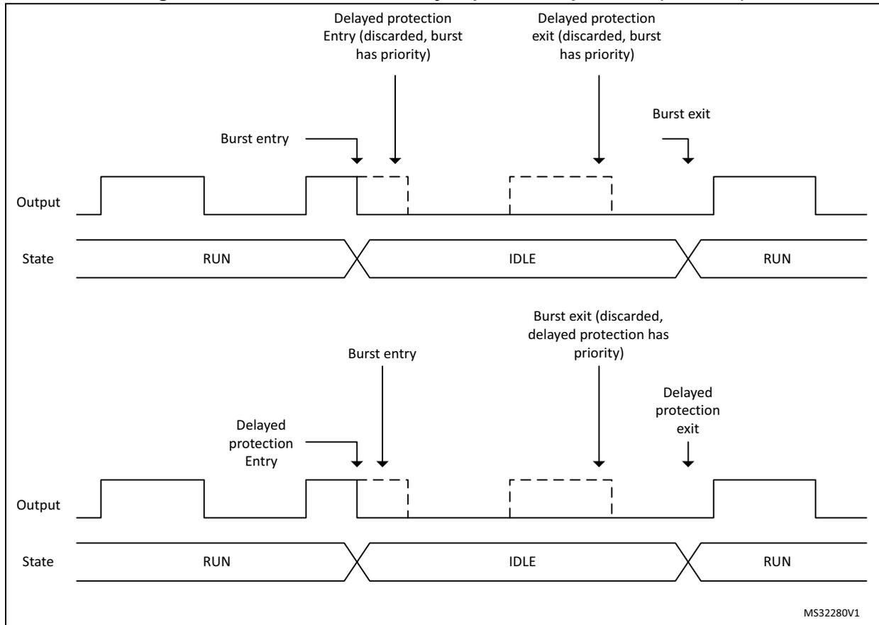
The same priorities are applied when the delayed burst mode entry is enabled (DIDL bit set), as shown on [Figure 278](#) below.
