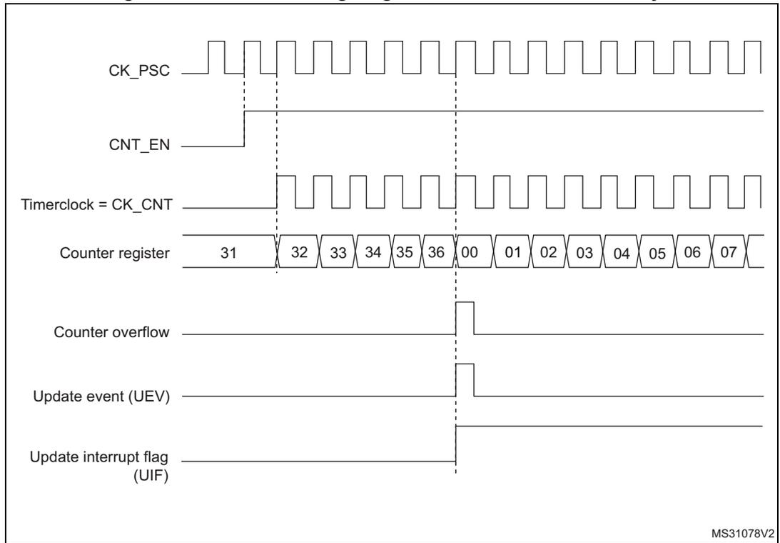
**Figure 217. Counter timing diagram, internal clock divided by 2**
