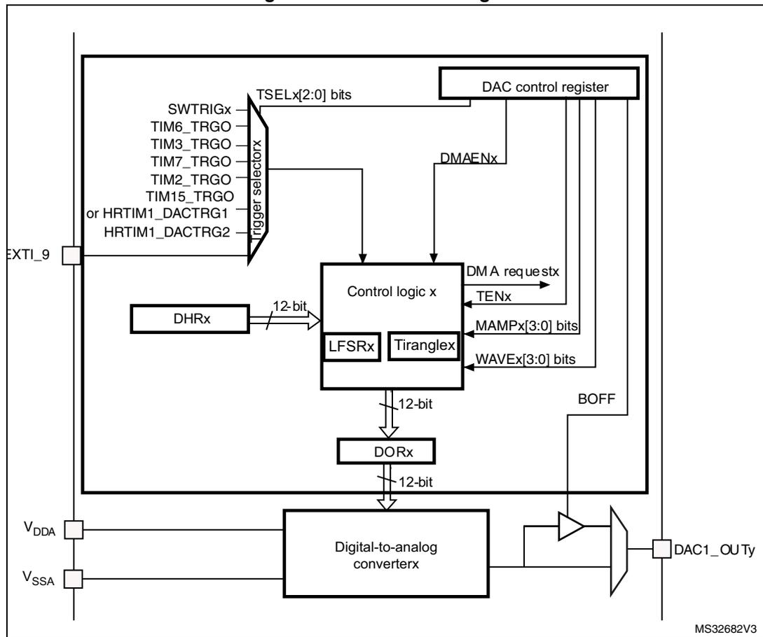
1. On STM32F334, there is no output buffer on the DAC1 channel 2. There is instead a switch allowing to connect the DAC1\_OUT2 to the corresponding I/O (PA5) (refer to DAC2 block diagram).
