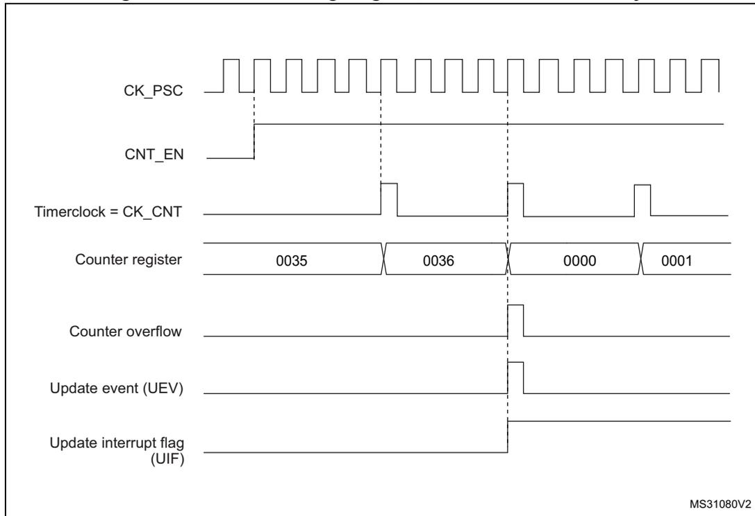
Figure 111. Counter timing diagram, internal clock divided by N
