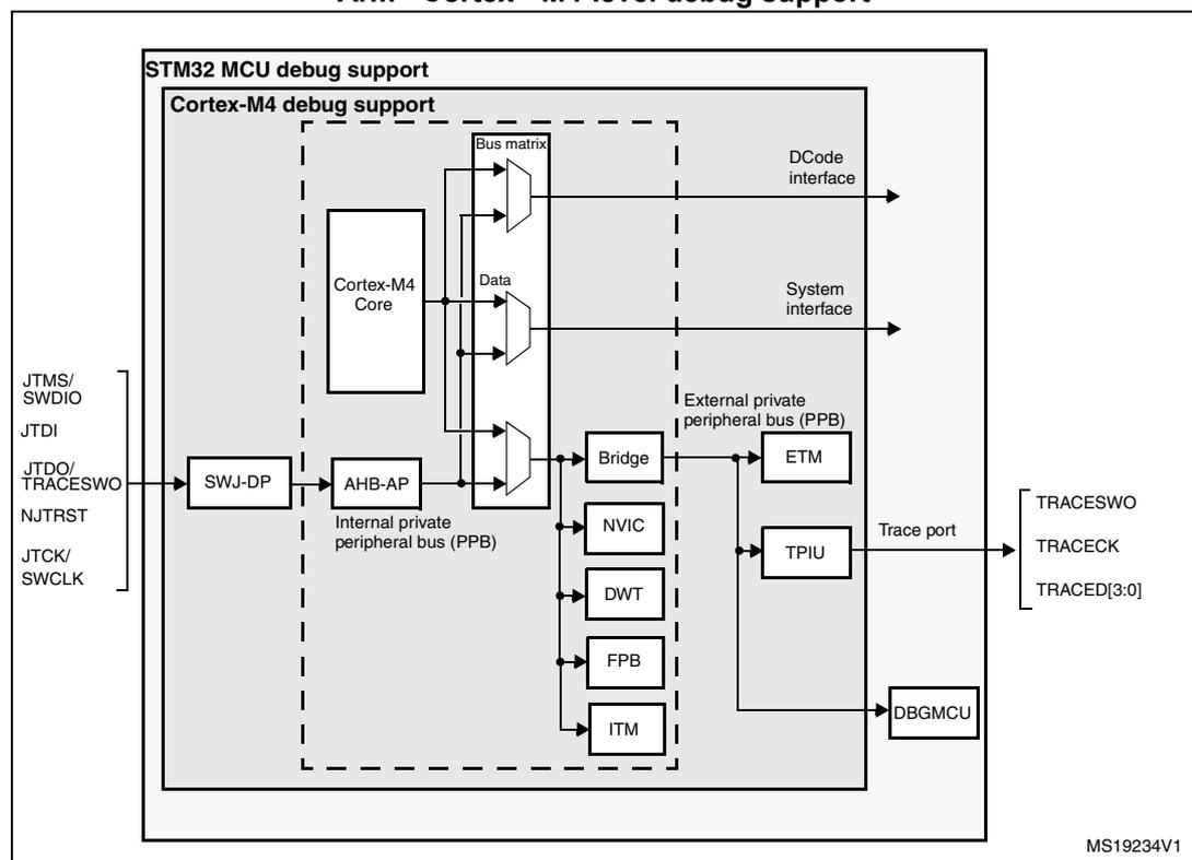
*Note:* The debug features embedded in the Cortex®-M4 core are a subset of the Arm® CoreSight Design Kit.
