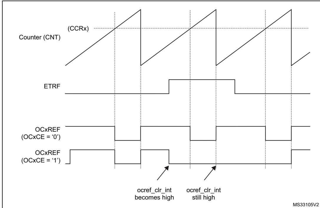
Note: In case of a PWM with a 100% duty cycle (if  $CCR_x > ARR$ ), OCxREF is enabled again at the next counter overflow.
