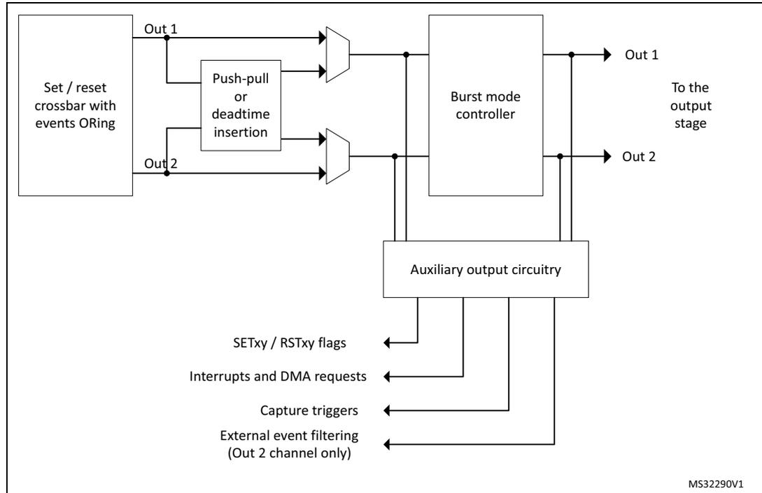
By default, the auxiliary outputs are copies of outputs Tx1 and Tx2. The exceptions are:
