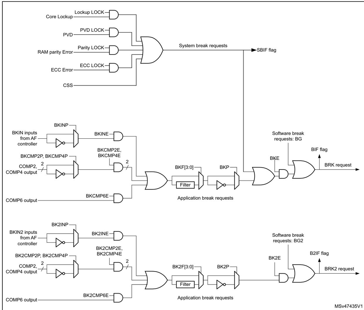
**Note:** An asynchronous (clockless) operation is only guaranteed when the programmable filter is disabled. If it is enabled, a fail safe clock mode (for example by using the internal PLL and/or the CSS) must be used to guarantee that break events are handled.
