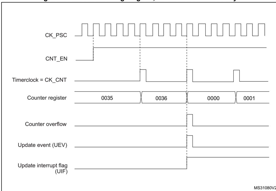
Figure 169. Counter timing diagram, internal clock divided by N
