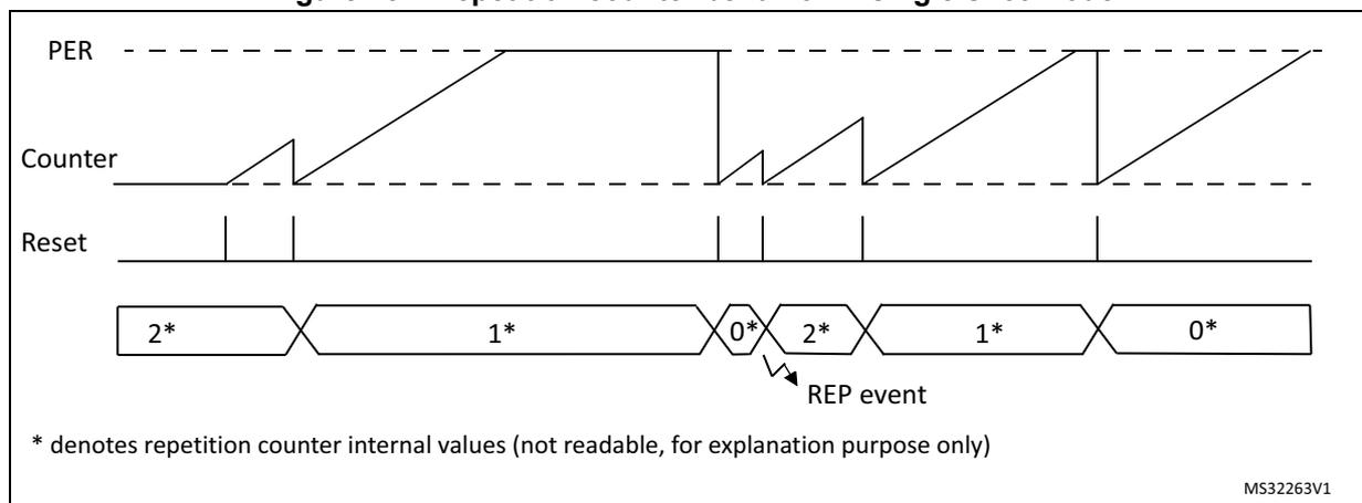
A reset or start event from the HRTIM\_SCIN[3:1] source causes the repetition to be decremented as any other reset. However, in SYNCIN-started single-shot mode (SYNCSTRTx bit set in the HRTIM\_TIMxCR register), the repetition counter will be decremented only on the 1st reset event following the period. Any subsequent reset will not alter the repetition counter until the counter is re-started by a new request on HRTIM\_SCIN[3:1] inputs.
