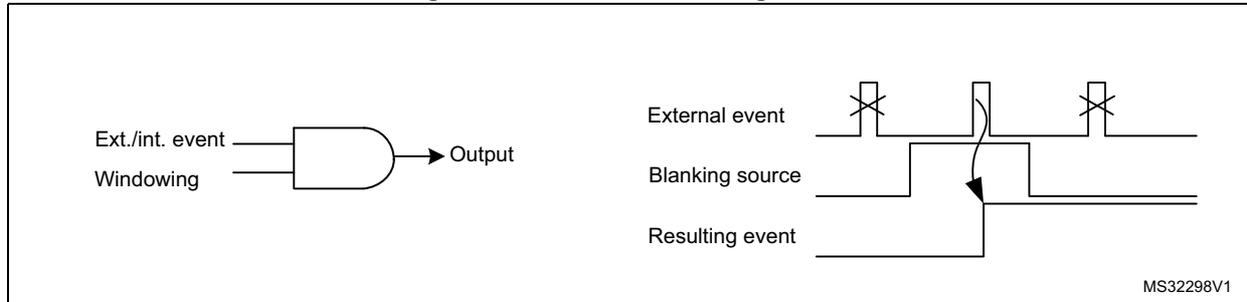
EExLTCH bit in EEFxR1 and EEFxR2 registers allows to latch the signal, if set to 1: in this case, an event is accepted if it occurs during the window but is delayed at the end of it.
