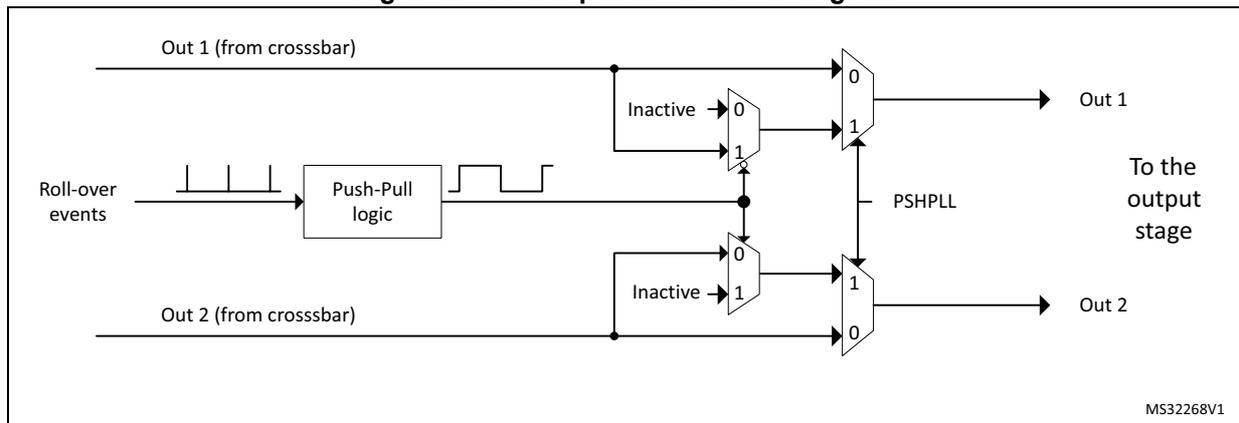
The push-pull mode is only available when the timer operates in continuous mode: the counter must not be reset once it has been enabled (TxCEN bit set). It is necessary to disable the timer to stop a push-pull operation and to reset the counter before re-enabling it.
