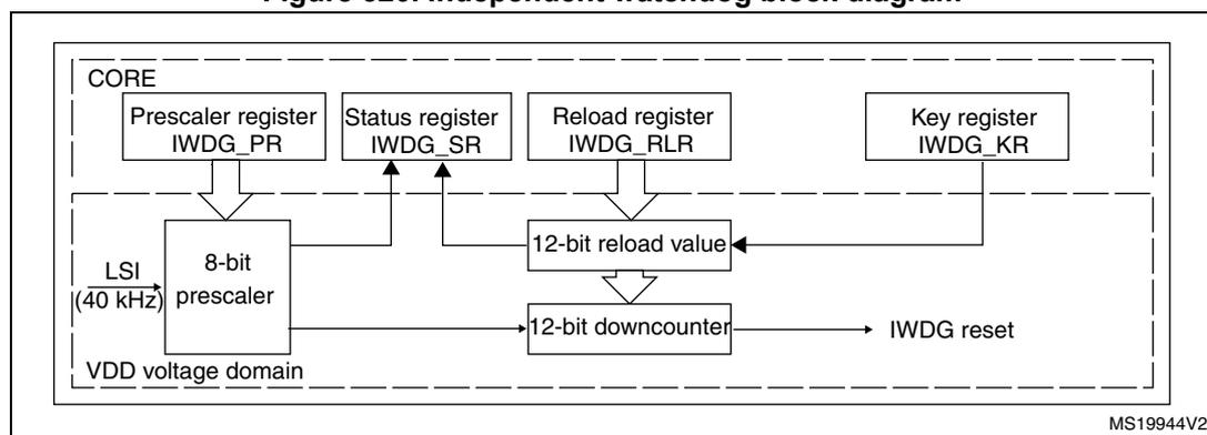
1. The watchdog function is implemented in the CORE voltage domain that is still functional in Stop and Standby modes.
