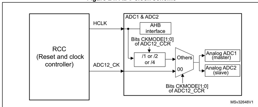
1. Refer to the RCC section to see how HCLK and ADC12\_CK can be generated.
