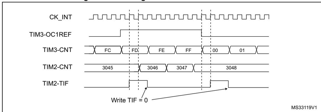
In the example in [Figure 207](#), the TIM2 counter and prescaler are not initialized before being started. So they start counting from their current value. It is possible to start from a given value by resetting both timers before starting TIM3. You can then write any value you want in the timer counters. The timers can easily be reset by software using the UG bit in the TIMx\_EGR registers.
