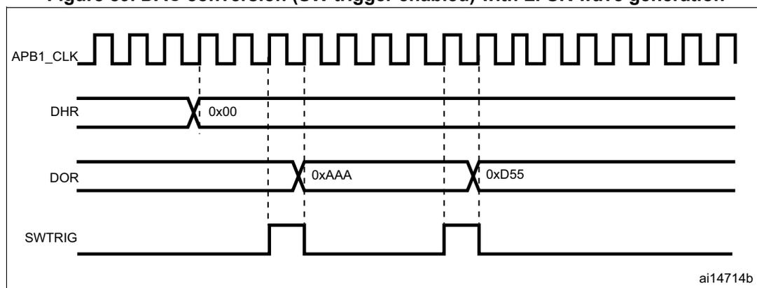
*Note:* The DAC trigger must be enabled for noise generation by setting the TENx bit in the DAC\_CR register.
