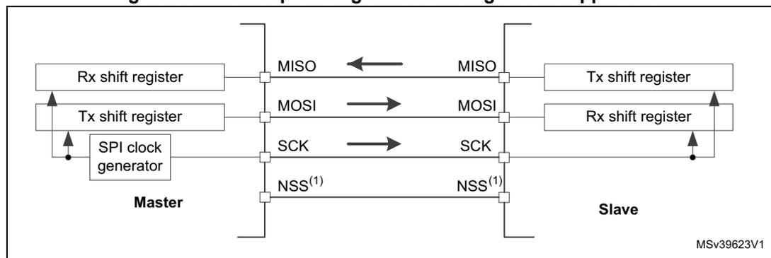
1. The NSS pins can be used to provide a hardware control flow between master and slave. Optionally, the pins can be left unused by the peripheral. Then the flow has to be handled internally for both master and slave. For more details see [Section 29.4.5: Slave select \(NSS\) pin management](#).
