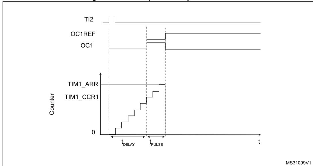
For example you may want to generate a positive pulse on OC1 with a length of t<sub>PULSE</sub> and after a delay of t<sub>DELAY</sub> as soon as a positive edge is detected on the TI2 input pin.
