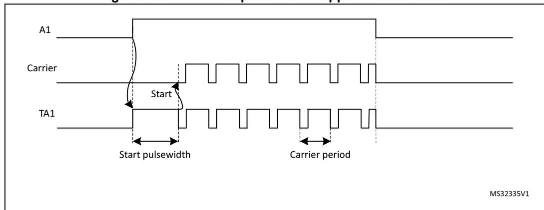
*Note:* **CHP1** and **CHP2** bits must be set prior to the output enable done with **TxyOEN** bits in the **HRTIM\_OENR** register.
