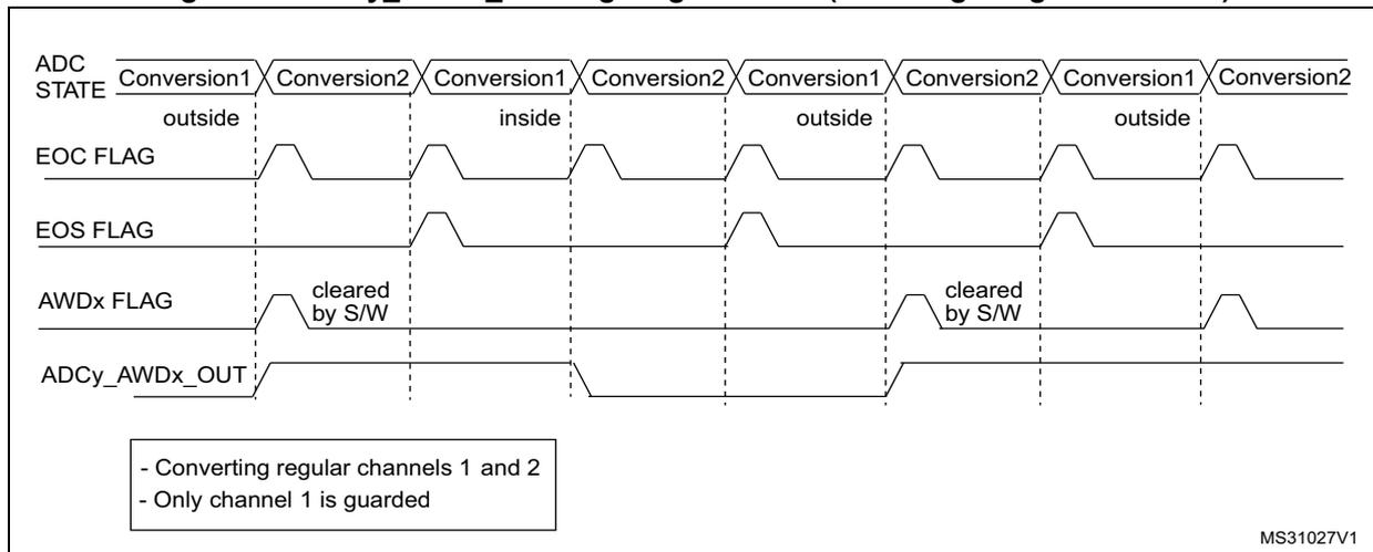
Figure 66. ADCy\_AWDx\_OUT signal generation (on all injected channels)
