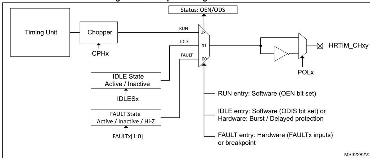
Figure 281 summarizes the bit values for the three states and how the transitions are triggered. Faults can be triggered by any external or internal fault source, as listed in Section 21.3.15, while the Idle state can be entered when the burst mode or delayed protections are active.
