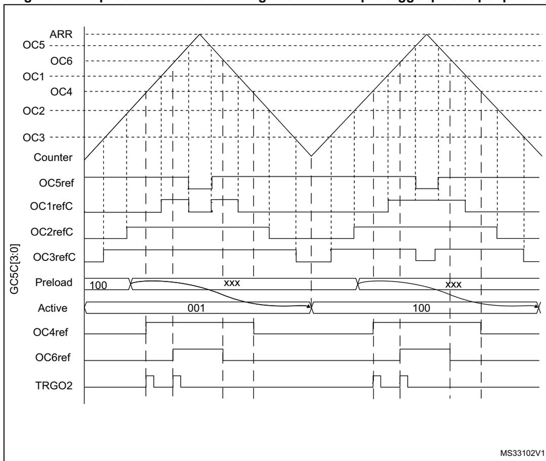
The TRGO2 waveform shows how the ADC can be synchronized on given 3-phase PWM signals. Please refer to [Section 18.3.26: ADC synchronization](#) for more details.
