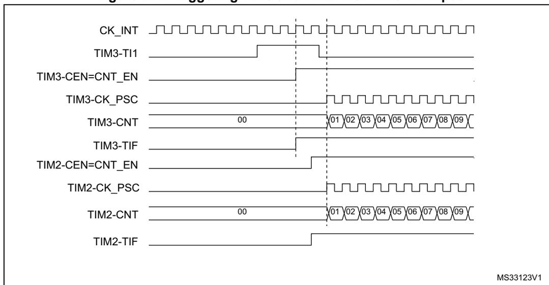
*Note:* The clock of the slave peripherals (timer, ADC, ...) receiving the TRGO or the TRGO2 signals must be enabled prior to receive events from the master timer, and the clock frequency (prescaler) must not be changed on-the-fly while triggers are received from the master timer.
