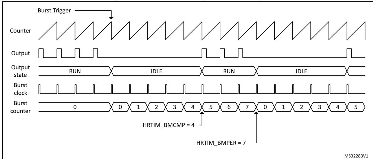
The burst mode controller consists of:
