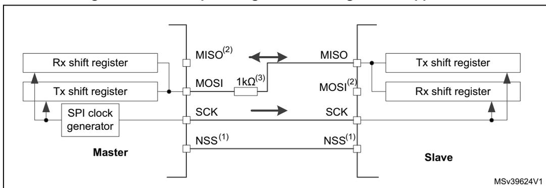
1. The NSS pins can be used to provide a hardware control flow between master and slave. Optionally, the pins can be left unused by the peripheral. Then the flow has to be handled internally for both master and slave. For more details see [Section 29.4.5: Slave select \(NSS\) pin management](#).
