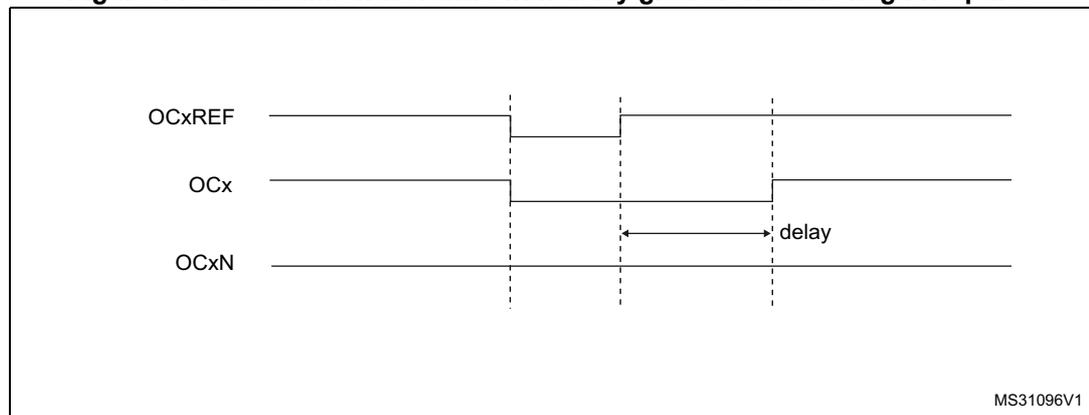
**Figure 146. Dead-time waveforms with delay greater than the positive pulse**
