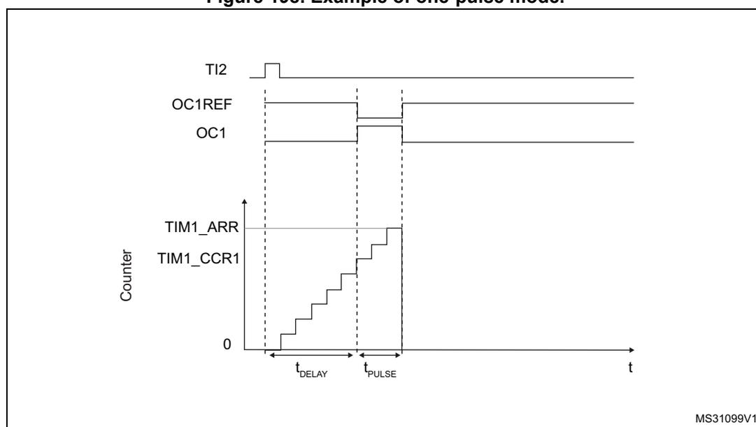
For example you may want to generate a positive pulse on OC1 with a length of  $t_{PULSE}$  and after a delay of  $t_{DELAY}$  as soon as a positive edge is detected on the TI2 input pin.
