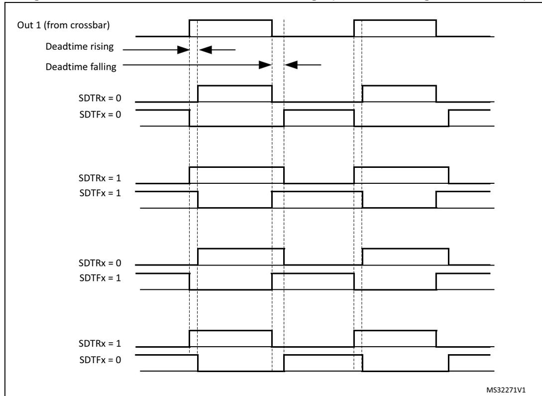
The deadtime values are defined with DTFx[8:0] and DTRx[8:0] bitfields and based on a specific clock prescaled according to DTPRSC[2:0] bits, as follows:
