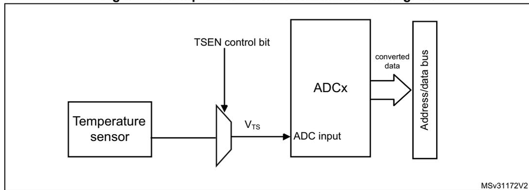
*Note:* The TSEN bit must be set to enable the conversion of the temperature sensor voltage  $V_{TS}$ .
