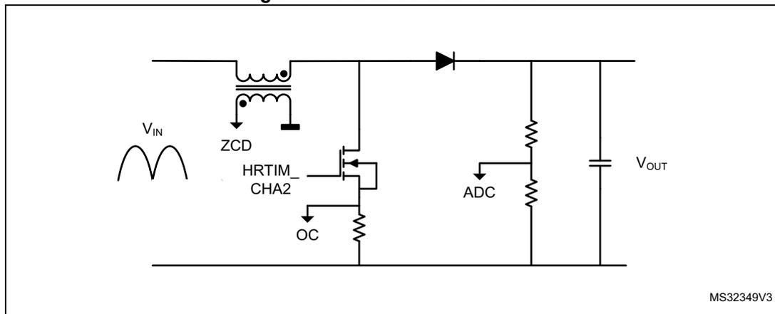
This converter is operating with a constant Ton time and a variable frequency due the Toff time variation (depending on the input voltage). It must also include some features to operate when no zero-crossing is detected, or to limit the Ton time in case of over-current (OC). The OC feedback is usually conditioned with the built-in comparator and routed onto an external event input.
