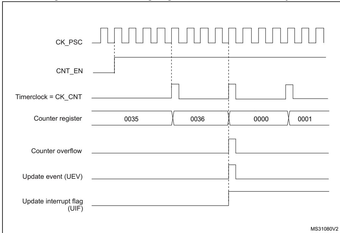
Figure 219. Counter timing diagram, internal clock divided by N
