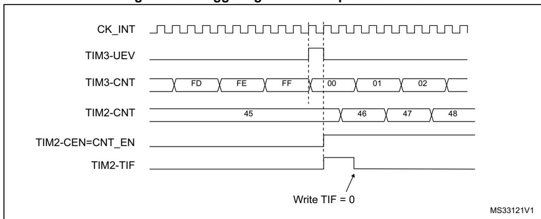
As in the previous example, you can initialize both counters before starting counting. [Figure 210](#) shows the behavior with the same configuration as in [Figure 209](#) but in trigger mode instead of gated mode (SMS=110 in the TIM2\_SMCR register).
