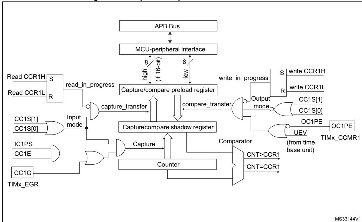
Figure 190. Output stage of capture/compare channel (channel 1)
