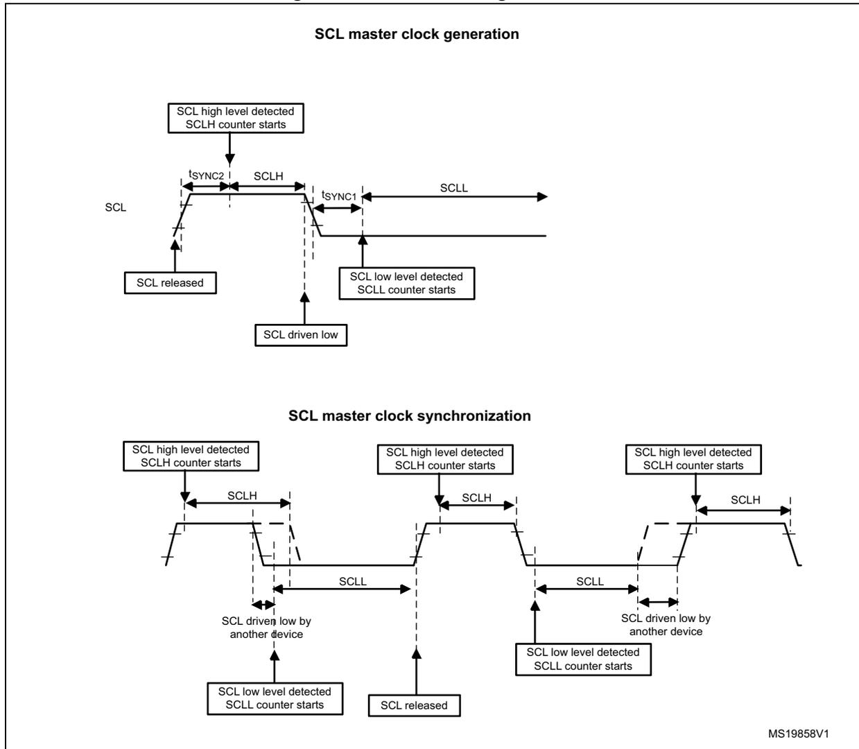
**Caution:** In order to be I<sup>2</sup>C or SMBus compliant, the master clock must respect the timings given below:
