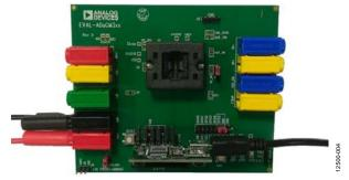
Figure 4. Mini-Link Debugger/Programmer Connection
