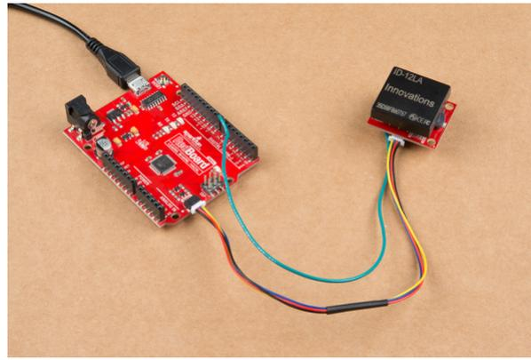
**Note:** The Qwiic system has a logic level of **3.3V**. I have attached the interrupt to pin 8 on the Redboard Qwiic even though the pin is at 5 volts. This will not harm the Qwiic RFID because we're doing a simple `digitalRead()` but also because the ATTiny84 is tolerant of voltages up to 5.5V.
