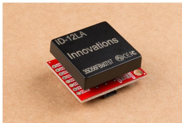
Each option is similar but there is a small variance in power consumption which translates into different read range capabilities. The ID-3LA is designed to be used with an external antenna which will get you 30cm of range. The ID-12LA and ID-20LA have a range of 12cm and 18cm respectively.
