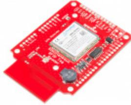
SparkFun Simultaneous RFID Reader - M6E Nano
